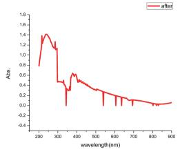
Fig. 16 UV-Visible spectra of the solution of 3.5% NaCl polluted by 16 ppm sulfide ions containing 300 ppm myrrh extract before and after 24 h of  $\alpha$ -brass immersion.
