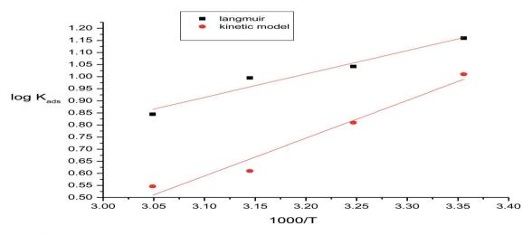
Fig. 5  $\log K_{\text{ads}}$  vs. (1/T) curves for the corrosion of  $\alpha$ -brass in 3.5% NaCl polluted by 16 ppm sulfide in the absence and presence of different concentrations of myrrh extract at different temperatures.
