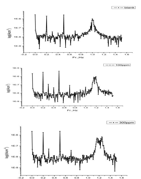
Fig. 12 EFM intermodulation spectra (current vs. frequency) without and with different concentrations of myrrh extract for corrosion of α-brass in 3.5% NaCl solution polluted at 25  $^{\circ}$ C.
