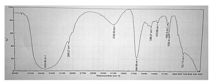
Fig. 14 FT-IR spectrum of the myrrh extract before adsorption on the  $\alpha$ -brass surface.
