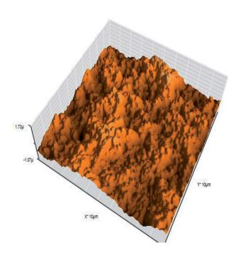
Fig. 13 (A) Surface of the  $\alpha$ -brass electrode imaged using atomic force microscopy after 24 h immersion in 3.5% NaCl solution polluted by 16 ppm sulfur ions. (B) Surface of the  $\alpha$ -brass electrode imaged using atomic force microscopy after 24 h immersion in 3.5% NaCl solution polluted by 16 ppm sulfur ions with 300 ppm myrrh extract.
