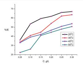
Fig. 2 The variation of inhibition efficiency with myrrh extract concentration of  $\alpha$ -brass in 3.5% NaCl + 16 ppm sulfide solutions.
