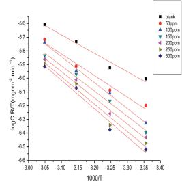
Fig. 7 Plots of log C.R./T vs. 1000/T for  $\alpha$ -brass in 3.5% NaCl polluted by 16 ppm sulfide without and with different concentrations of myrrh extract at 25 °C.
