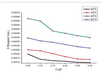
Fig. 1 Corrosion rates of various concentrations of myrrh extract on  $\alpha$ -brass in 3.5% NaCl + 16 ppm sulfide at 25–55 °C.
