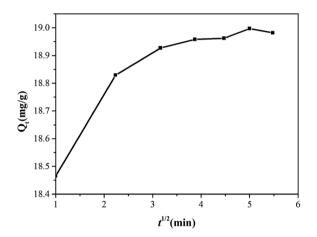
Fig. 11 Plot of intraparticle diffusion model for the adsorption of  $Cr^{6+}$  by  $Zn(\shortparallel)$  dithiocarbamate/ZnS nanocomposite.
