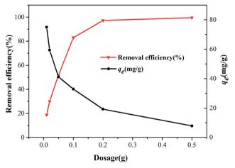
Fig. 7 Effect of dosage on the  $Cr^{6+}$  removal efficiency of  $Zn(\shortparallel)$  dithiocarbamate/ZnS nanocomposite (conditions: 20 mL medium; 200 mg  $L^{-1}$  initial concentration of  $Cr^{6+}$ ; pH=4.5; 10 min contact time: 293 K).
