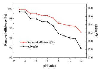
Fig. 8 Effect of pH value on the removal efficiency (conditions: 20 mL medium; 200 mg  $L^{-1}$  initial concentration of  $Cr^{6+}$ ; 0.2 g dosage; 10 min contact time; 293 K).
