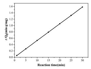
Fig. 10 Pseudo second-order kinetic model of adsorption for  $Cr^{6+}$  by Zn(III) dithiocarbamate/ZnS nanocomposite.
