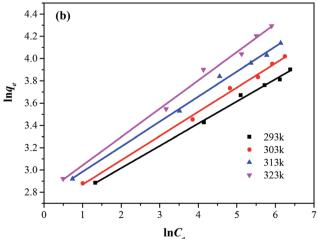
Fig. 13 (a) Langmuir adsorption isotherms and (b) Freundlich adsorption isotherms at 293 K, 303 K, 313 K and 323 K respectively.
