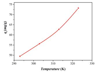
Fig. 9 Effect of temperature on the removal efficiency (conditions: 20 mL medium; 200 mg  $L^{-1}$  initial concentration of  $Cr^{6+}$ ; 0.2 g dosage; pH = 4.5; 10 min contact time).
