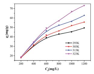
Fig. 12 Adsorption isotherm of Cr<sup>6+</sup> initial concentration.
