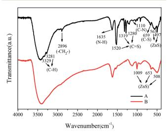
Fig. 2 (A) FTIR spectra of Zn(III) dithiocarbamate/ZnS nanocomposite and (B) FTIR spectra of nanoparticles after adsorption reaction.
