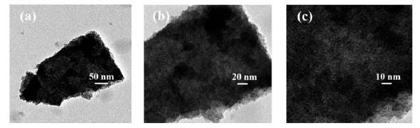
Fig. 5 TEM images of Zn(II) dithiocarbamate/ZnS nanocomposite.
