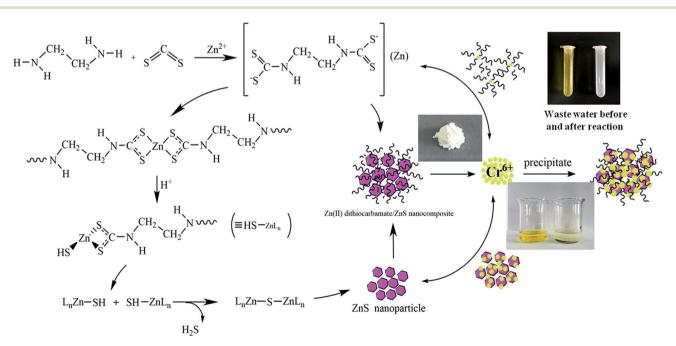
Reaction mechanism during the Cr<sup>6+</sup> removal.
