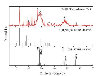
Fig. 6 XRD patterns of Zn(II) dithiocarbamate/ZnS nanocomposite.
