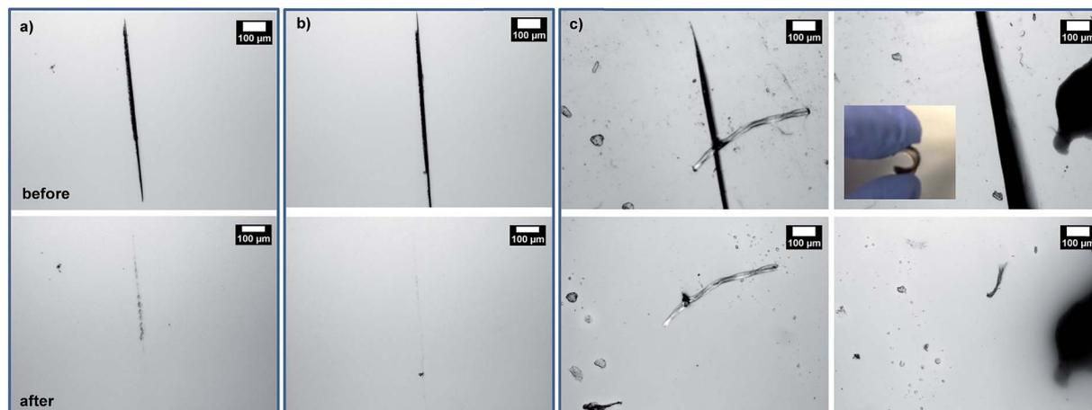
Fig. 5 Optical microscope images of cuts on DA-crosslinked F1M1 (a), F2M1 (b), and F3M1 (c) films before and after being annealed at 150 °C for 5 h and following 80 °C for 2 h. Inset of (c) digital image of F3M1 film.
