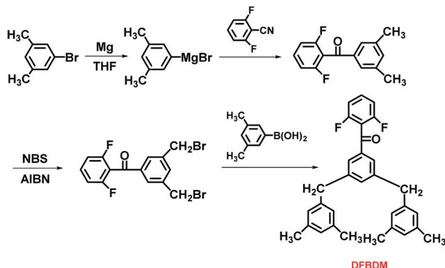
Fig. 1 Synthetic route of difluoro monomer DFBDM.
