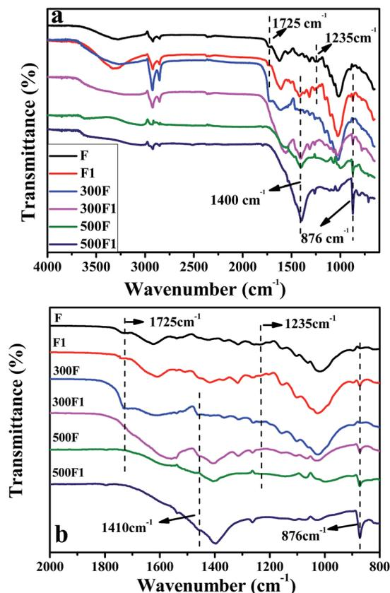
Fig. 1 FTIR spectra of the untreated hemp fiber F and treated hemp fiber F1, the thermal degradation residue 300F, 300F1, 500F and 500F1 (a); the enlarged spectra range of  $750\text{--}2500 \text{ cm}^{-1}$  (b).
