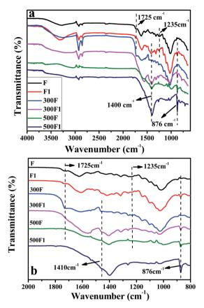
Fig. 1 FTIR spectra of the untreated hemp fiber F and treated hemp fiber F1, the thermal degradation residue 300F, 300F1, 500F and 500F1 (a); the enlarged spectra range of  $750-2500 \text{ cm}^{-1}$  (b).
