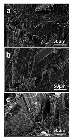
Fig. 6 SEM photos of the fractured composite surface: (a) PPF-50, (b) PPF1-50, (c) PPF1-50-15R composite.
