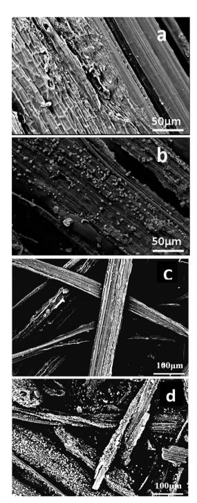
Fig. 2 SEM photos of the hemp fiber surface: (a) F; (b) F1, and the thermal degradation residue of hemp fiber surface: (c) 500F, (d) 500F1.
