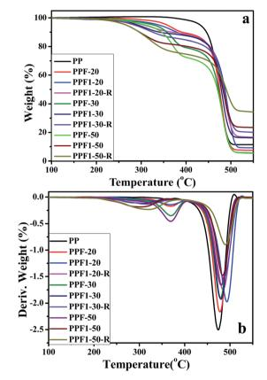
Fig. 8 (a) TGA thermograms of pure PP and the composites; (b) DTG curves of pure PP and the composites.
