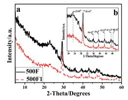
Fig. 3 WAXD curves of the 500F and 500F1 (a); the enlarged specta of the region 30 < 2-theta < 50 degrees (b).
