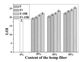
Fig. 4 Limiting oxygen index of the treated and untreated hemp and their reinforced composites.
