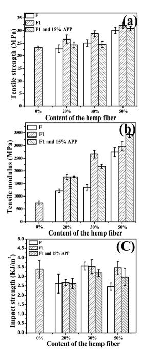
Fig. 5 Effect of hemp fiber loading ratio on the tensile strength (a), tensile modulus (b) of hemp fiber/PP composites and (c) impact strength.
