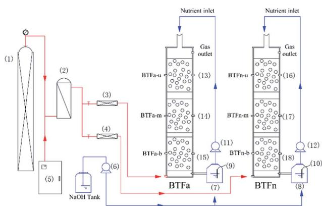
Fig. 1 Schematic diagram of the biotrickling filter (1) H<sub>2</sub>S cylinder, (2) mixing chamber, (3 and 4) gas flowmeter, (5) air compressor, (6) NaOH dosing pump, (7 and 8) nutrient tank, (9 and 10) pH probe, (11 and 12) peristaltic pump, (13–15) filter material sampling sites, (16–18) air sampling ports.
