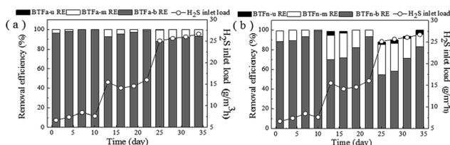
Fig. 2 H<sub>2</sub>S removal profiles of the BTFa (a) and the BTFn (b).
