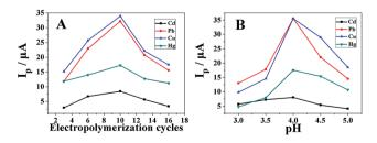
Fig. 6 DPASV carried out on the polyfurfural film/MWCNTs/GCE with coexistent 10  $\mu g~L^{-1}~Cd^{2+}$ , 10  $\mu g~L^{-1}~Pb^{2+}$ , 10  $\mu g~L^{-1}~Cu^{2+}$ , and 10  $\mu g~L^{-1}~Hg^{2+}$  in 0.1 M acetate buffer solution with different numbers of electropolymerization cycles of furfural (A) and different pH values (B) (deposition potential: -1.2 V, deposition time: 300 s).
