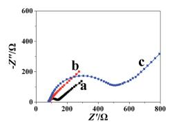
Fig. 1 EIS of (a) bare GCE, (b) MWCNTs/GCE, and (c) polyfurfural film/MWCNTs/GCE in 5.0 mM  $\rm K_3[Fe(CN)_6]/K_4[Fe(CN)_6]$  solution containing 0.1 M KCl.
