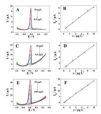
Fig. 4 DPASV curves of Pb<sup>2+</sup> at different concentrations at the (A) polyfurfural film/GCE, (C) MWCNTs/GCE, and (E) polyfurfural film/MWCNTs/GCE in 0.1 M acetate buffer solution (pH 4.0). Linear relationship between anodic stripping peak current and concentration at (B) polyfurfural film/GCE, (D) MWCNTs/GCE, and (F) polyfurfural film/MWCNTs/GCE.
