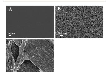
Fig. 2 SEM images of (A) bare GCE, (B) MWCNTs/GCE and (C) polyfurfural film/MWCNTs/GCE.
