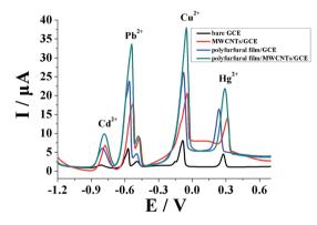
Fig. 5 DPASV curves for bare GCE, MWCNTs/GCE, polyfurfural film/GCE, and polyfurfural film/MWCNTs/GCE in coexistent 10  $\mu g \, L^{-1} \, Cd^{2+},$  10  $\mu g \, L^{-1} \, Pb^{2+},$  10  $\mu g \, L^{-1} \, Cu^{2+},$  and 10  $\mu g \, L^{-1} \, Hg^{2+}$  in 0.1 M acetate buffer solution (pH 4.0). Electropolymerization cycles of furfural: 10 cycles, pH: 4.0, deposition potential: -1.2 V, deposition time: 300 s.
