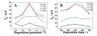
Fig. 7 DPASV carried out on the polyfurfural film/MWCNTs/GCE in coexistent 10  $\mu$ g L<sup>-1</sup> Cd<sup>2+</sup>, 10  $\mu$ g L<sup>-1</sup> Pb<sup>2+</sup>, 10  $\mu$ g L<sup>-1</sup> Cu<sup>2+</sup>, and 10  $\mu$ g L<sup>-1</sup> Hg<sup>2+</sup> in 0.1 M acetate buffer solution with different deposition potentials (A) and different deposition times (B) (electropolymerization cycles of furfural: 10 cycles, pH: 4.0).
