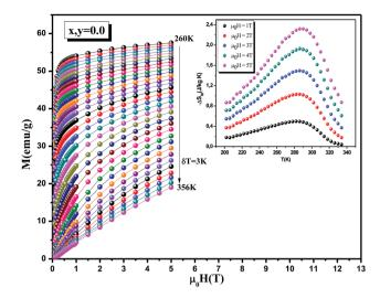
Fig. 2 Magnetic field dependence of magnetization at several temperatures for La $_{0.7}$ Ca $_{0.1}$ Pb $_{0.2}$ Mn $_{1-x-y}$ Al $_x$ Sn $_y$ O $_3$  (x,y=0.0) sample, the inset: temperature dependence of the magnetic entropy change ( $-\Delta S_{\rm M}$ ) at different applied magnetic field change intervals for La $_{0.7}$ Ca $_{0.1}$ Pb $_{0.2}$ Mn $_{1-x-y}$ Al $_x$ Sn $_y$ O $_3$  (x,y=0.05).
