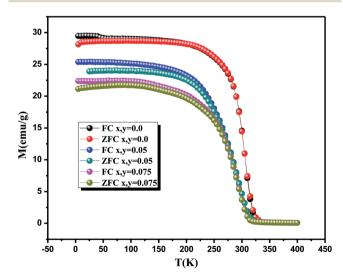
**Fig. 1** Temperature dependences of ZFC and FC magnetization for  $La_{0.7}Ca_{0.1}Pb_{0.2}Mn_{1-x-y}Al_xSn_yO_3$  (x, y = 0.0, 0.05 and 0.075) compounds under a magnetic field of 0.05 T.
