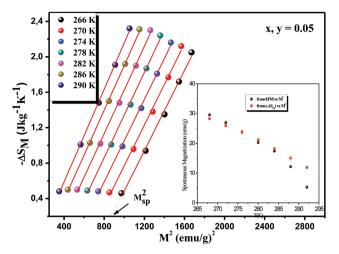
Fig. 14 Isothermal  $-\Delta S_M$  vs.  $M^2$  curves (the solid lines are linear fits to the data). The inset: spontaneous magnetization of La<sub>0.7</sub>Ca<sub>0.1</sub>Pb<sub>0.2</sub>-Mn<sub>0.9</sub>Al<sub>0.05</sub>Sn<sub>0.05</sub>O<sub>3</sub> deduced from the extrapolation of the isothermal  $-\Delta S_M$  vs.  $M^2$  curves and from the Arrott plots  $\mu_0 H/M$  vs.  $M^2$ .
