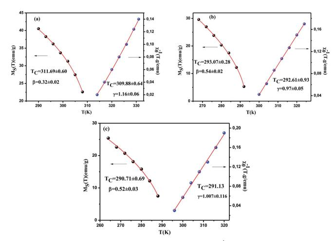
Fig. 8 The spontaneous magnetization  $M_S(T, 0)$  (left) and the inverse initial susceptibility  $\chi_0^{-1}(T)$  (right) as a function of temperature of La<sub>0.7</sub>- $Ca_{0.1}Pb_{0.2}Mn_{0.9}Al_{0.05}Sn_{0.05}O_3$ , (a) for x, y = 0.0, (b) for x, y = 0.05 and x, y = 0.075.
