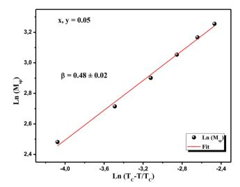
Fig. 15 Ln  $(M_{Sp})$  vs. Ln  $(T_C - T/T_C)$ . The red line is the linear fitting.
