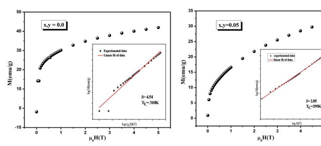
Fig. 10 Critical isotherms of *M versus*  $\mu_0 H$  for La<sub>0.7</sub>Ca<sub>0.1</sub>Pb<sub>0.2</sub>Mn<sub>1-x-y</sub>Al<sub>x</sub>Sn<sub>y</sub>O<sub>3</sub> (x, y=0.0 and 0.05). The inset: shows the log-log scale for *M versus*  $\mu_0 H$ .
