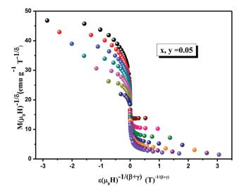
Fig. 13 Normalized isotherms of  $La_{0.7}Ca_{0.1}Pb_{0.2}Mn_{0.9}Al_{0.05}Sn_{0.05}O_3$  below and above the Curie temperature using the values of  $\beta$  and  $\Delta$  determined by the K–F method.
