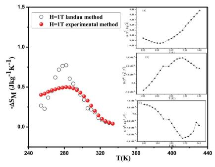
Fig. 3 Experimental and calculated values of the magnetic entropy change vs. temperature used the Landau theory under applied magnetic field of 1 T for the  $La_{0.7}Ca_{0.1}Pb_{0.2}Mn_{0.9}Al_{0.05}Sn_{0.05}O_3$  compound. The inset: (a)–(c): variation of Landau parameters A, B and C as a function of temperature of  $La_{0.7}Ca_{0.1}Pb_{0.2}Mn_{0.9}Al_{0.05}Sn_{0.05}O_3$ .
