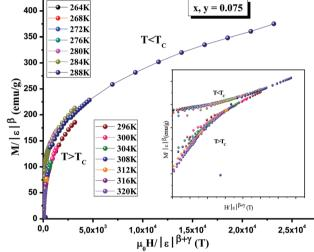
Fig. 12 Scaling plots for La $_{0.7}$ Ca $_{0.1}$ Pb $_{0.2}$ Mn $_{1-x-y}$ Al $_x$ Sn $_y$ O $_3$  (x, y=0.0 and 0.075) below and above  $T_C$  using  $\beta$  and  $\gamma$  determined by the Kouvel–Fisher method. The insets show the same plots on a log–log scale.
