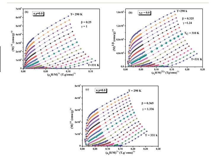
Fig. 6 Modified Arrott plots:  $M^{1/\beta}$  versus ( $\mu_0 H/M$ )<sup>1/ $\gamma$ </sup> with (a) tricritical mean-field model ( $\beta=0.25, \gamma=1$ ), (b) 3D-Ising model ( $\beta=0.325, \gamma=1.24$ ) and (c) 3D-Heisenberg model ( $\beta=0.365, \gamma=1.336$ ).
