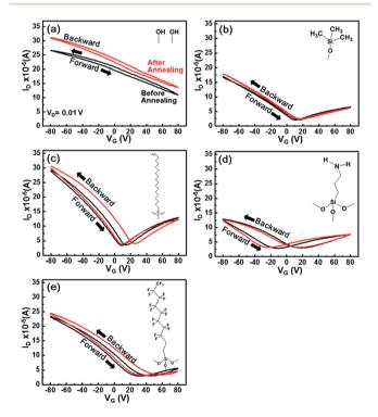
Fig. 3 Transfer curves of graphene transistors on various SAMs-modified SiO<sub>2</sub>/Si substrates before (black line) and after annealing at 100 °C (red line): (a) SiO<sub>2</sub>/Si, (b) HMDS, (c) ODTS, (d) APS, and (e) FDTS. Bias of  $V_{\rm GS}=-80$  V and  $V_{\rm DS}=0.01$  V were applied on the graphene transistors.
