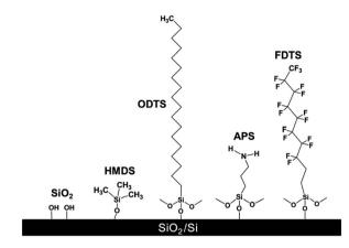
Fig. 1 Schematics of self-assembled monomers (SAMs) on SiO<sub>2</sub>/Si substrates. SiO<sub>2</sub>: untreated SiO<sub>2</sub>/Si, HMDS: hexamethyldisilazane treated, ODTS: octadecyltrichlorosilane treated, APS: 3-aminopropyltriethoxysilane treated, and FDTS: 1H,1H,2H,2H-perfluorodecyltriethoxysilane treated
