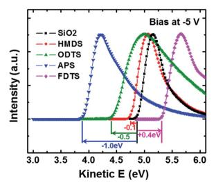
Fig. 2 Secondary electron emission spectra of the SiO<sub>2</sub>/Si substrates treated with various SAMs
