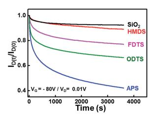
Fig. 4 Bias stability of graphene transistors with various SAMs-modified  $SiO_2/Si$  substrates. Bias of  $V_{GS}=-80$  V and  $V_{DS}=0.01$  V were applied on the graphene transistors for 60 min.
