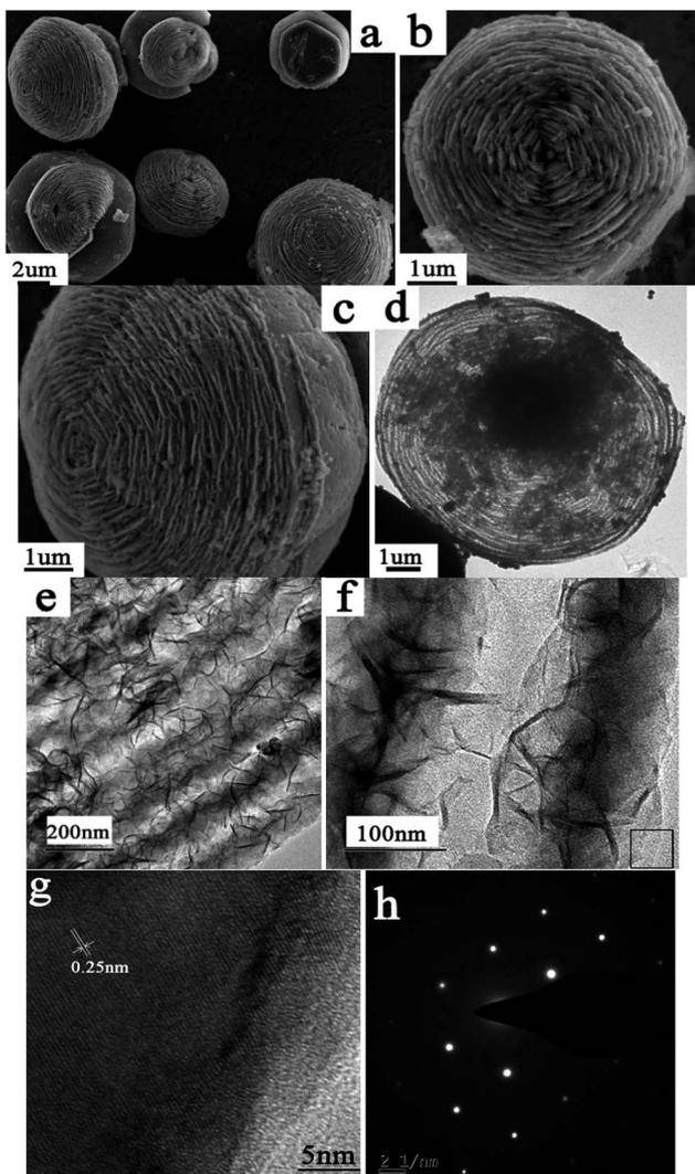
Fig. 2 SEM (a–c), TEM (c–f), HRTEM (g) and SAED (h) images of the ZnO obtained in the typical process.
