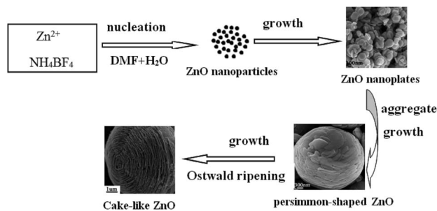
Scheme 1 Illustration of the growth process of hierarchical cake-like ZnO microstructures.
