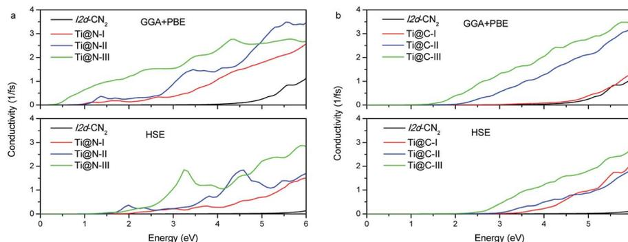
Fig. 7 Photoconductivity of (a) Ti@N and (b) Ti@C.
