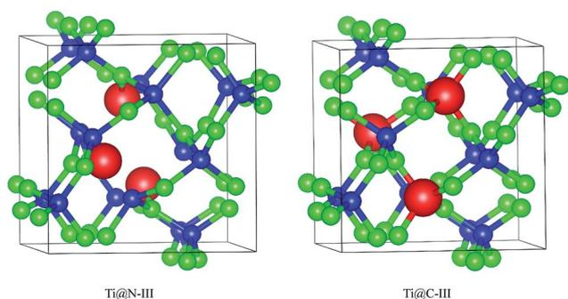
Fig. 1 Doped I2d-CN<sub>2</sub> structures with substitution of N and C by three Ti atoms.
