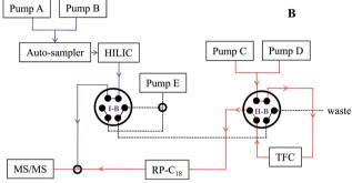
Fig. 1 Brief schematic of HILIC-TFC-RPLC-MS/MS platform: (A), loading phase (0–4.0 min) and (B), parallel elution phase (4.0–32.0 min). The details in regard of the operation principles can be found in Section "2.4 Configuration of HILIC-TFC-RPLC-MS/MS".
