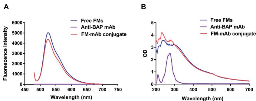
**Fig. 3** (A). Fluorescence intensities of free FMs, anti-BAP mAb and FM-mAb conjugates. (B). Ultraviolet visible spectra of FMs, anti-BAP mAb and FM-mAb conjugates.
