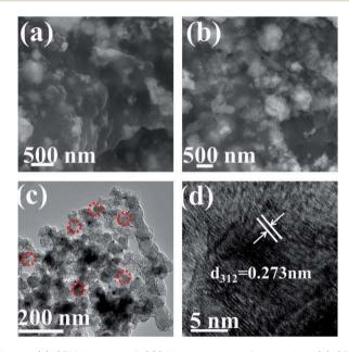
Fig. 5 (a) SEM images of CS24 electrodes before cycles, (b) SEM images of CS24 electrodes after 10 discharge/charge cycles at a current density of 50 mA  $g^{-1}$ , and (c) low-magnification TEM image showing well-maintained morphology of CS24 electrode after discharge to 0.05 V, and (d) high-magnification TEM displaying details of CS24 electrode after discharge to 0.05 V at a current density of 50 mA  $g^{-1}$ .
