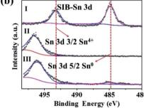
Fig. 4 XPS spectra of Cu2p and Sn3d for (I) the pristine CuSn alloy, (II) the electrode of the first discharge to  $0.05\ V$  before etching, (III) the electrode of the first discharge to  $0.05\ V$  after 2 min of argon etching.
