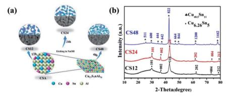
Fig. 1 (a) Schematic for the fabrication procedure of the CSA nanoporous composites. (b) XRD patterns of CSA nanoporous composites with different corrosion time (in 1 M NaOH aqueous solution).
