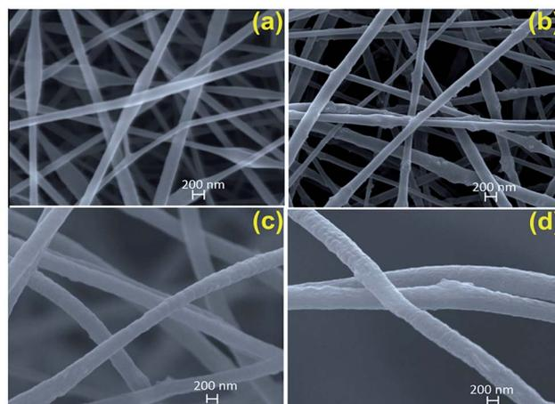
Fig. 4 SEM images of (a) pristine PAN nanofiber, (b) PAN/TiO<sub>2</sub> nanofiber, (c) PAN/ZnO and (d) TiO<sub>2</sub>/ZnO/PAN nanofibers.
