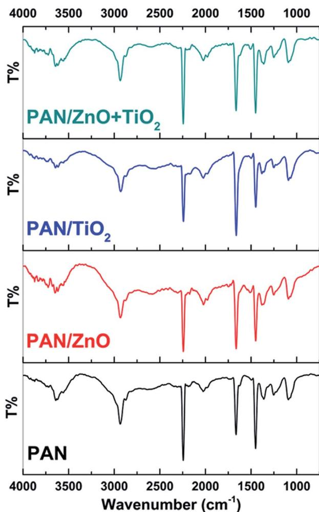
Fig. 8 FTIR spectra of pristine PAN nanofiber, PAN/TiO<sub>2</sub> nanofiber, PAN/ZnO and PAN/ZnO-TiO<sub>2</sub> nanofibers.
