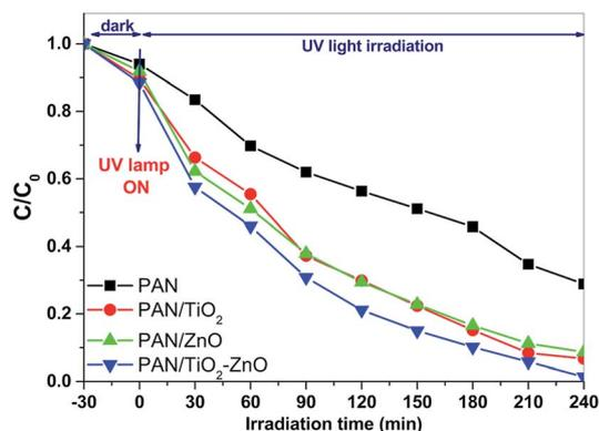
Fig. 10 Decolorization comparison of the MG with respect to time intervals over electrospun PAN, PAN/ $\text{TiO}_2$ , PAN/ $\text{ZnO}$  and  $\text{TiO}_2/\text{ZnO}/\text{PAN}$  photocatalyst under UV light (catalyst concentration:  $0.3 \text{ mg mL}^{-1}$ ; initial concentration of dye:  $1.0 \times 10^{-5} \text{ M}$ ).
