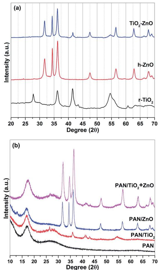
Fig. 2 XRD patterns of (a) nanostructures prepared *via* arc-discharge method showing rutile structure of TiO<sub>2</sub>, hexagonal wurtzite structure of ZnO and TiO<sub>2</sub>-ZnO nanocomposite structures, (b) PAN based nanocomposite electrospun fibers.
