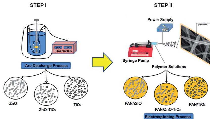
Fig. 1 The methodology used to fabricate PAN based electrospun fibers modified with ZnO, TiO<sub>2</sub> and ZnO–TiO<sub>2</sub> nanostructures.
