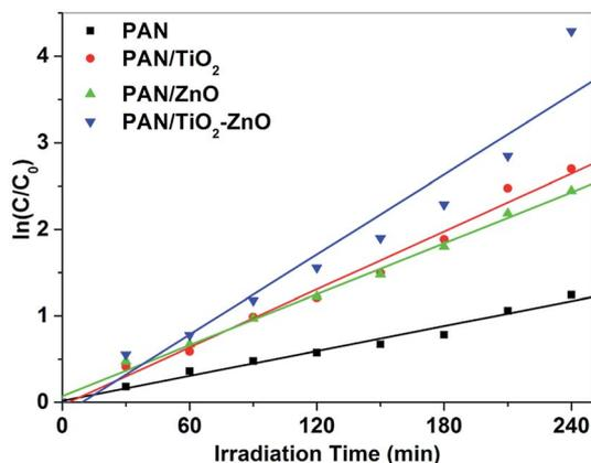
Fig. 11 Comparison of the apparent rate constants of electrospun PAN, PAN/ $\text{TiO}_2$ , PAN/ $\text{ZnO}$  and  $\text{TiO}_2/\text{ZnO}/\text{PAN}$  photocatalysts under UV light irradiation (catalyst concentration:  $0.3 \text{ mg mL}^{-1}$ ; initial concentration of dyes:  $1.0 \times 10^{-5} \text{ M}$ ).
