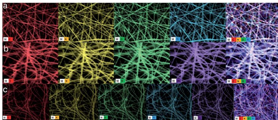
Fig. 5 Elemental mapping images of (a) PAN/TiO<sub>2</sub> nanofiber, (b) PAN/ZnO and (c) TiO<sub>2</sub>/ZnO/PAN nanofibers.
