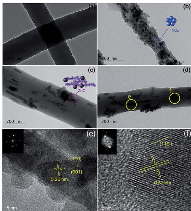
Fig. 6 TEM images of (a) pristine PAN nanofiber, (b) PAN/TiO<sub>2</sub> nanofiber, (c) PAN/ZnO and (d) TiO<sub>2</sub>/ZnO/PAN nanofibers, HR-TEM image of TiO<sub>2</sub>/ZnO/PAN hybrid nanofibers marked from yellow circle of (d) and the upper left inset the corresponding SAED pattern (e and f).
