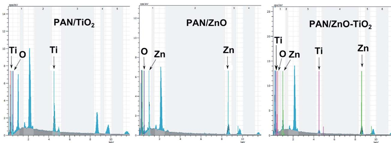
Fig. 7 EDX spectra of electrospun PAN based nanofibers containing TiO<sub>2</sub>, ZnO and TiO<sub>2</sub>-ZnO.
