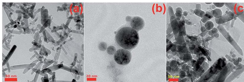
Fig. 3 Representative TEM images of (a) ZnO nanoparticles (scale bar 50 nm), (b)  $\alpha$ -TiO<sub>2</sub> nanospheres (scale bar 20 nm), (c) ZnO + TiO<sub>2</sub> nanocomposite structures (scale bar 50 nm).
