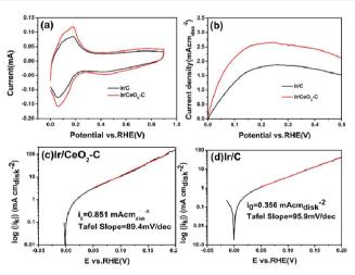
Fig. 6 (a) Cyclic voltammograms of 10% Ir/CeO<sub>2</sub>-C and 10% Ir/C catalysts (Ar-saturated 0.1 M KOH, 50 mV s<sup>-1</sup>, room temperature). (b) Linear scanning voltammograms of 10% Ir/CeO2-C and 10% Ir/C catalysts (H<sub>2</sub>-saturated 0.1 M KOH, 10 mV s<sup>-1</sup>, 1600 rpm, room temperature). Tafel plot of (c) 10% Ir/CeO<sub>2</sub>-C catalyst and (d) 10% Ir/C catalyst.
