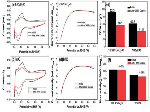
Fig. 7 Cyclic voltammogram of (a) Ir/CeO<sub>2</sub>-C and (b) Ir/C before and after 2000 potential cycles. Linear scanning voltammograms of (c) Ir/ CeO2-C and (d) Ir/C before and after 2000 potential cycles. ECSA (e) and mass activity@ 50 mV (f) of Ir/CeO2-C and Ir/C before and after 2000 cycles.
