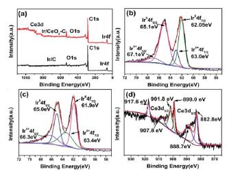
Fig. 5 XPS analysis of (a) 10% Ir/CeO<sub>2</sub>-C and 10% Ir/C full XPS spectrum; (b) Ir 4f spectrum of 10% Ir/C, (c) Ir 4f spectrum of 10% Ir/CeO<sub>2</sub>-C, and (d) Ce 3d spectrum of 10%  $Ir/CeO_2-C$ .
