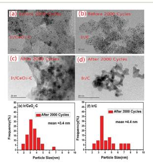
Fig. 8 TEM images and particle size distribution histograms of 10% Ir/  $CeO_2-C$  (a, c, and e) and 10% Ir/C (b, d, and f) catalysts before and after 2000 potential cycles.
