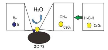
Schematic of 10% Ir/CeO<sub>2</sub>-C for HOR in a basic solution.
