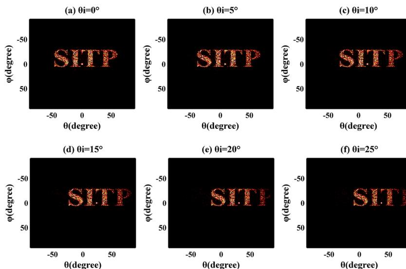
Fig. 5 Imaging dependence on the incidence angle. Far field intensities for the metasurface hologram simulated with incident angle (a)  $0^\circ$ , (b)  $5^\circ$ , (c)  $10^\circ$ , (d)  $15^\circ$ , (e)  $20^\circ$ , (f)  $25^\circ$ , at designed wavelength.
