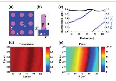
Fig. 1 Schematic structure of metasurface with periodic  $TiO_2$  nanodisks (H = 650 nm, P = 245 nm). (a) Top view. (b) Side view. (c) Numerically calculated transmission (black triangle) and phase shift (blue square) for metasurfaces with varied radius and fixed period P = 245 nm at wavelength  $\lambda = 560$  nm. Transmittance and transmitted light phase variation as a function of TiO<sub>2</sub> nanodisk radius (R) and period (P) are shown in (d) and (e), respectively.
