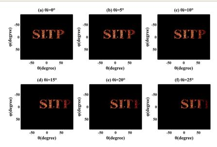
Fig. 5 Imaging dependence on the incidence angle. Far field intensities for the metasurface hologram simulated with incident angle (a) 0°, (b) 5°, (c)  $10^{\circ}$ , (d)  $15^{\circ}$ , (e)  $20^{\circ}$ , (f)  $25^{\circ}$ , at designed wavelength.
