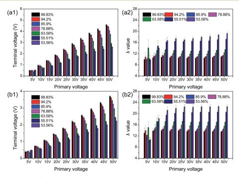
Fig. 3 Changes in terminal voltage ( $U'_S$ ) and  $\lambda$  ( $U_P/U'_S$ ) determined by transformer 18 as affected by primary voltage at frequencies of 400 Hz and 700 Hz; (a1) terminal voltage, 400 Hz; (a2) λ value, 400 Hz; (b1) terminal voltage, 700 Hz; (b2) λ value, 700 Hz.
