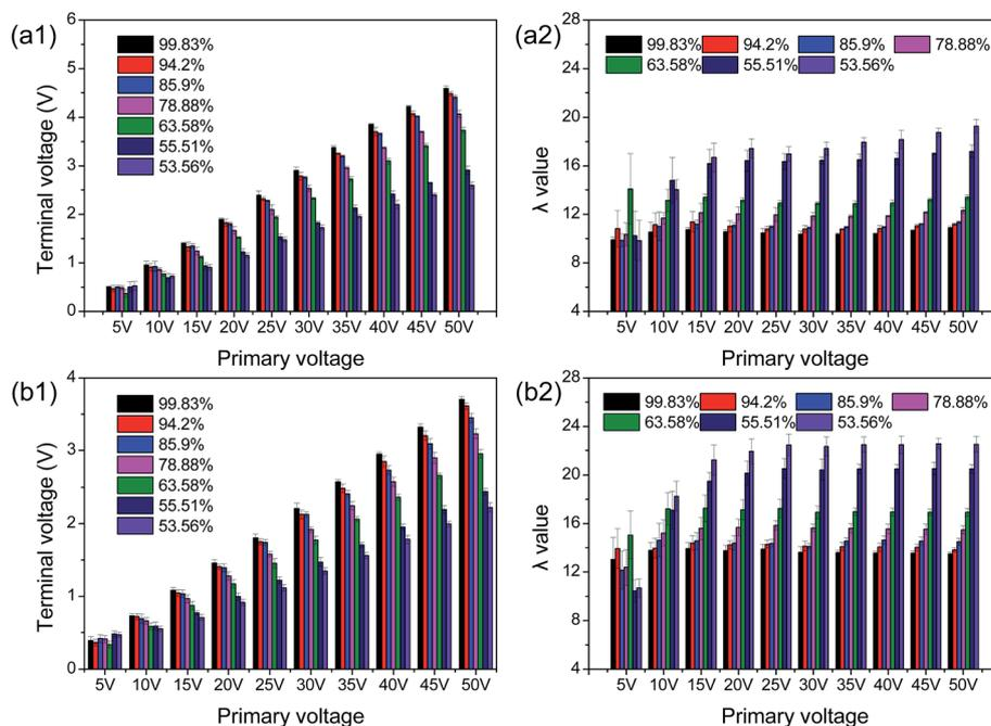
Fig. 3 Changes in terminal voltage ( $U'_S$ ) and  $\lambda$  ( $U_p/U'_S$ ) determined by transformer 18 as affected by primary voltage at frequencies of 400 Hz and 700 Hz: (a1) terminal voltage, 400 Hz; (a2)  $\lambda$  value, 400 Hz; (b1) terminal voltage, 700 Hz; (b2)  $\lambda$  value, 700 Hz.
