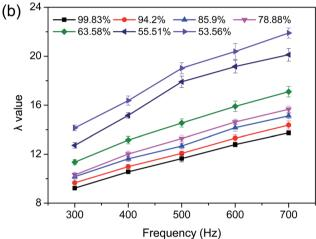
Fig. 2 Effects of frequency and DD on induced-electrical parameters determined by *transformer 18* at 20 V primary voltage ( $U_P$ ): (a) terminal voltage ( $U_S$ ); (b)  $\lambda$  value ( $U_P/U_S$ ).
