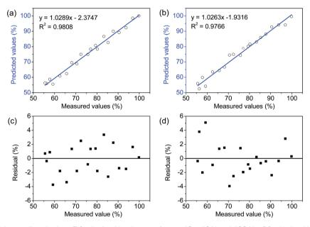
Fig. 4 Correlation plot of the predicted values ((a): obtained by the  $transformer\ 18$  at 10 V and 400 Hz; (b): obtained by  $transformer\ 100$  at 10 V and 400 Hz) and the residual values ((c): calculated from the regression model obtained by  $transformer\ 18$  at 10 V and 700 Hz; (d): calculated from the regression model obtained by  $transformer\ 100$  at 10 V and 400 Hz)  $transformer\ 100$  at 10 V and 400 Hz  $transformer\ 100$  at 10 V and 400 Hz tran
