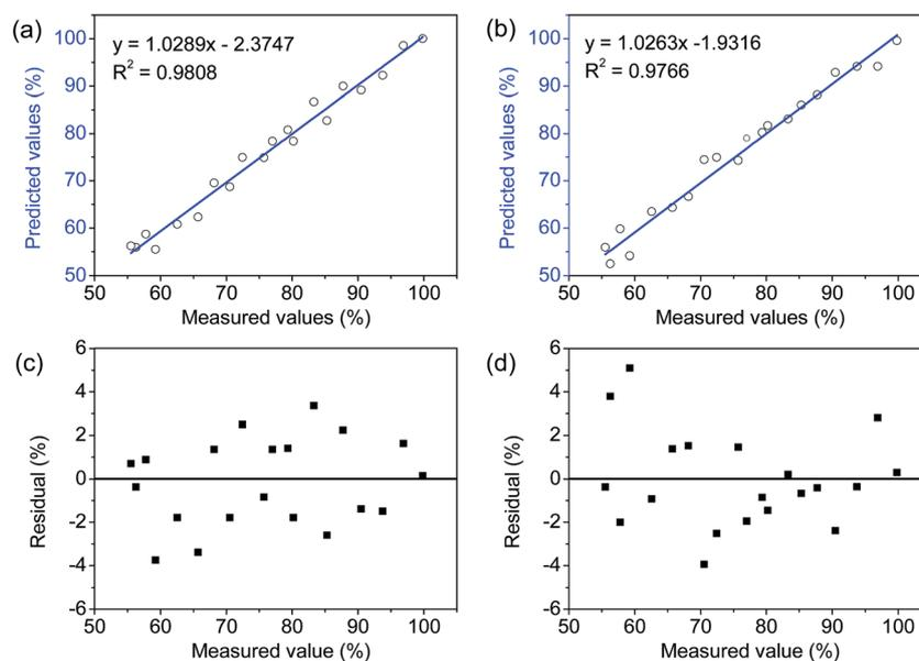
Fig. 4 Correlation plot of the predicted values ((a): obtained by the *transformer 18* at 10 V and 400 Hz; (b): obtained by *transformer 100* at 10 V and 400 Hz) and the residual values ((c): calculated from the regression model obtained by *transformer 18* at 10 V and 700 Hz; (d): calculated from the regression model obtained by *transformer 100* at 10 V and 400 Hz) versus the measured DD.
