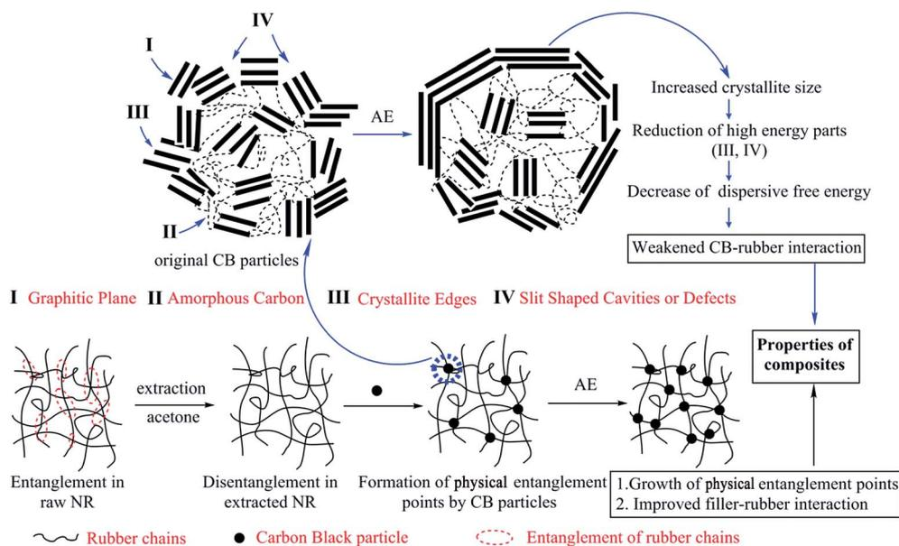
Fig. 11 Mechanism of CB–rubber interaction influenced by AE.
