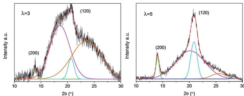
Fig. 7 XRD crystallization peak fitting of NR/CB composites without AE at different strain.
