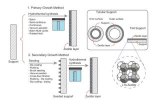
Fig. 3 Schematic of LTA zeolite membrane preparation methods.
