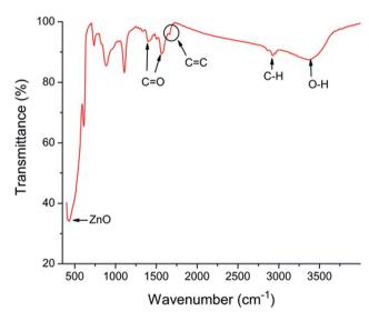
Fig. 4 FT-IR spectrum of the stationary phase.
