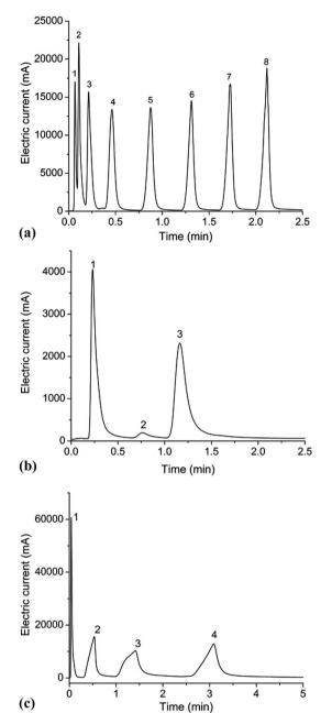
Fig. 5 Separations of the mixture of eight alkanes (a), three ester components (b), and four alcohols (c) by the RGO/ZnO column. The gas from component 1 to 8 in (a) is pentane, hexane, octane, nonane, decane, undecane and dodecane, respectively. The gas from component 1 to 3 in (b) is butyl acetate, ethyl lactate and ethyl heptanoate, respectively. The gas from component 1 to 4 in (c) is butyl alcohol, hexanol, octanol and lauryl alcohol, respectively.
