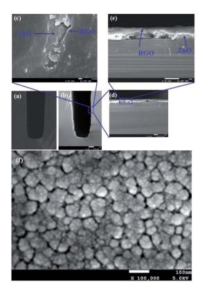
Fig. 3 SEM images of bare MEMS-based column channel (a), RGO/ZnO bilayer coated channel (b), the surface of the bilayer coating (c), the cross section of bilayer coating with 8000 times (d), 20 000 times (e), and surface morphology of ZnO underlayer (f).
