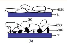
Fig. 2 Schematic diagram of single-layer stationary phase (a) and bilayer stationary phase (b).
