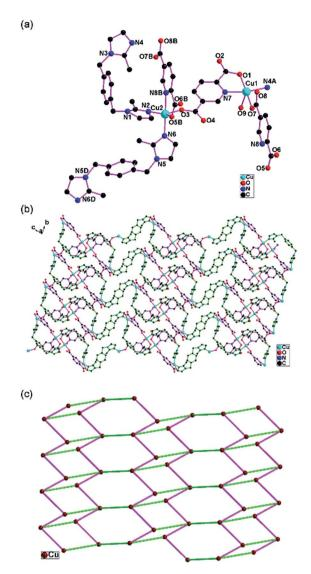
Fig. 5 (a) The coordination environment of Cu(ii) atom in 5; (b) the 2D network in 5; (c) the (3,4)-connected 2D network in 5. The pink and bright green sticks exhibit the 2,5-pydc and bix ligands, respectively. The pink and bright green sticks exhibit the 2,5-pydc and bix ligands.
