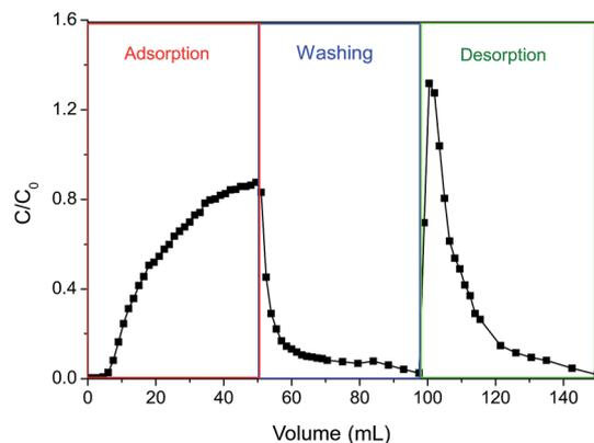
Fig. 7 The dynamic adsorption and desorption curve of poly-(DMAEMA)-grafted EVAL membrane (EVAL<sub>10</sub>, 0.6 mg BSA per mL, pH 6.4, 10 mM PBS,  $3.8 \text{ L m}^{-2} \text{ h}^{-1}$ ).
