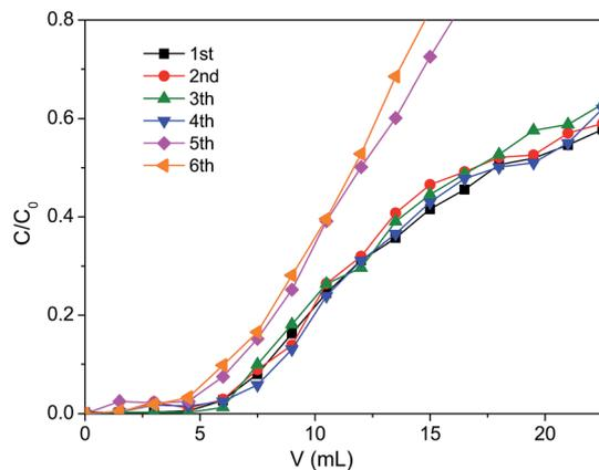
Fig. 9 The effect of adsorption/desorption cycle numbers on dynamic adsorption of membrane EVAL<sub>10</sub> (EVAL<sub>10</sub>, 0.6 mg BSA per mL, pH 6.4, 10 mM PBS).
