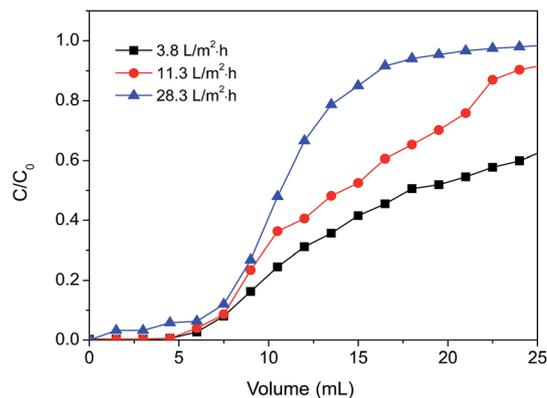
Fig. 10 The effect of flow rate on dynamic protein adsorption of poly(DMAEMA)-grafted EVAL membrane (EVAL<sub>10</sub>, 0.6 mg BSA per mL, pH 6.4, 10 mM PBS).
