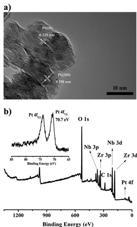
Fig. 6 (a) TEM image of Pt/Nb<sub>5</sub>Zr<sub>5</sub>-550 catalyst. (b) XPS survey spectrum of Pt/Nb<sub>5</sub>Zr<sub>5</sub>-550 catalyst (the insert is Pt XPS peaks).
