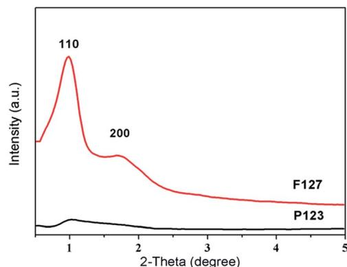
Fig. 1 Small-angle XRD patterns of Nb<sub>5</sub>Zr<sub>5</sub>-550 sample by using different templates.
