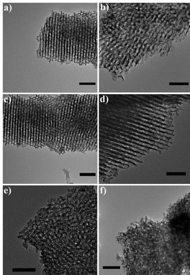
Fig. 3 TEM images of the mesoporous  $\text{Nb}_{10-x}\text{Zr}_x\text{-550}$  samples using F127: (a)  $\text{Nb}_5\text{Zr}_5$ , (b)  $\text{Nb}_6\text{Zr}_4$ , (c)  $\text{Nb}_7\text{Zr}_3$ , (d)  $\text{Nb}_8\text{Zr}_2$ , (e)  $\text{Nb}_9\text{Zr}_1$ , (f) Nb (scale bar: 50 nm).
