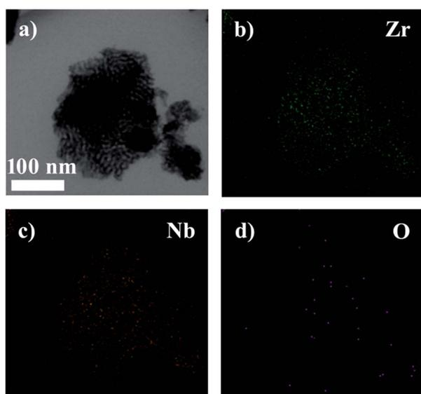
Fig. 4 HAADF-STEM image (a) and the corresponding elemental mapping images of the mesoporous Nb<sub>5</sub>Zr<sub>5</sub>-550 sample using F127: (b) elemental mapping of Zr; (c) elemental mapping of Nb; (d) elemental mapping of O (scale bar: 100 nm).
