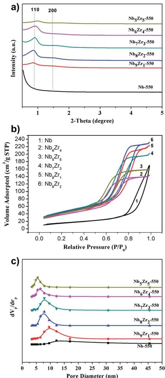
Fig. 2 (a) Small-angle XRD patterns of  $\text{Nb}_{10-x}\text{Zr}_x\text{-550}$  samples with different ratio of niobium to zirconium using F127. (b)  $\text{N}_2$  sorption isotherms of the  $\text{Nb}_{10-x}\text{Zr}_x\text{-550}$  samples using F127. (c) Pore size distribution curves of the  $\text{Nb}_{10-x}\text{Zr}_x\text{-550}$  samples using F127.
