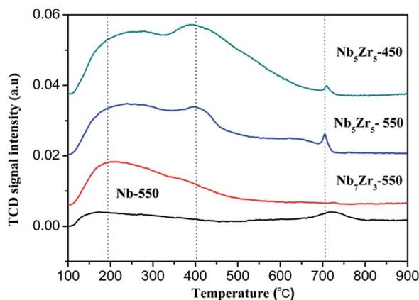
Fig. 5 NH<sub>3</sub>-TPD curves of Nb<sub>10-x</sub>Zr<sub>x</sub> mixed oxides using F127.
