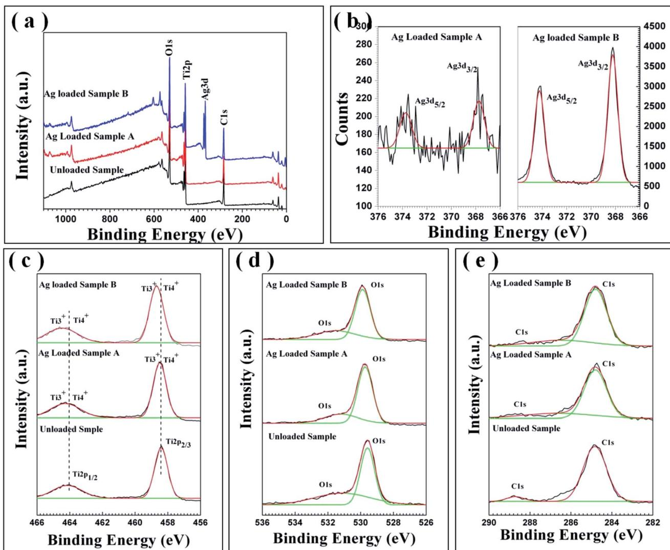
**Fig. 6** XPS survey spectrum (a) and high-resolution XPS spectrum of Ag 3d (b), Ti 2p (c), O 1s (d) and C 1s (e) of the Ag loaded samples and unloaded  $\text{TiO}_2$  mesoporous nanofibers for comparison.
