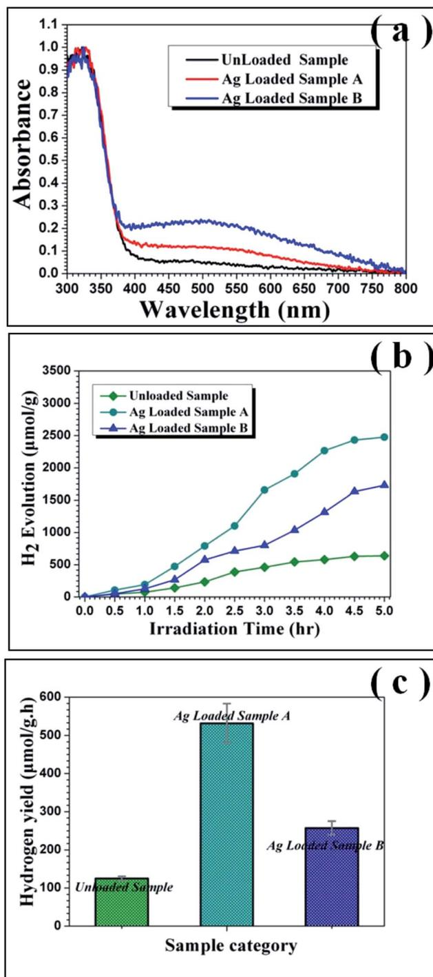
Fig. 7 (a) UV-vis diffuse reflectance absorption spectra of the as-synthesized Ag@TiO<sub>2</sub> mesoporous nanofibers and unloaded TiO<sub>2</sub> mesoporous products. (b) Hydrogen production photocatalysed by the as-fabricated Ag@TiO<sub>2</sub> mesoporous nanofibers and unloaded TiO<sub>2</sub> samples under different irradiation time. (c) Dependence of the TBOT concentration on the photocatalytic activity of resultant TiO<sub>2</sub> nanostructures for hydrogen evolution.
