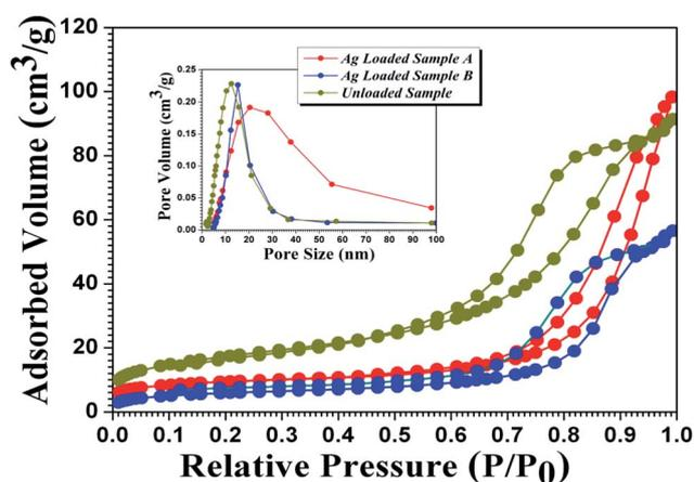
Fig. 5 N<sub>2</sub> adsorption and desorption isotherm of unloaded TiO<sub>2</sub> mesoporous nanofibers and Ag loaded samples. The inset is the corresponding pore size distribution of the three products.
