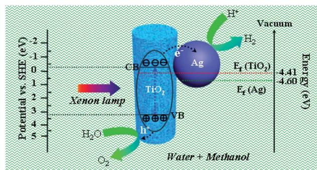
Fig. 8 Schematic diagram illustrating the possible photocatalytic mechanism of the Ag@TiO<sub>2</sub> mesoporous nanofibers under xenon lamp irradiation.
