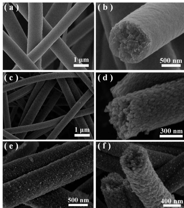
Fig. 2 (a and b) Typical SEM images of the as-spun polymer precursor for sample B and pure TiO<sub>2</sub> Sample. (c and d) Representative SEM images under different magnifications of the corresponding calcined products for unloaded Sample. (e and f) Representative SEM images of the as-prepared loaded sample B under different magnifications.
