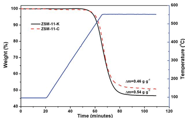
Fig. 7 TG profiles of the used catalysts.
