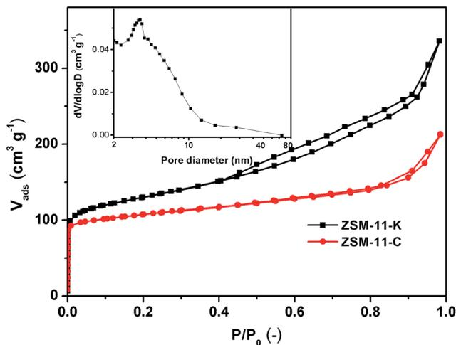
Fig. 3  $N_2$  isotherms and BJH pore size distributions of ZSM-11-C and ZSM-11-K.
