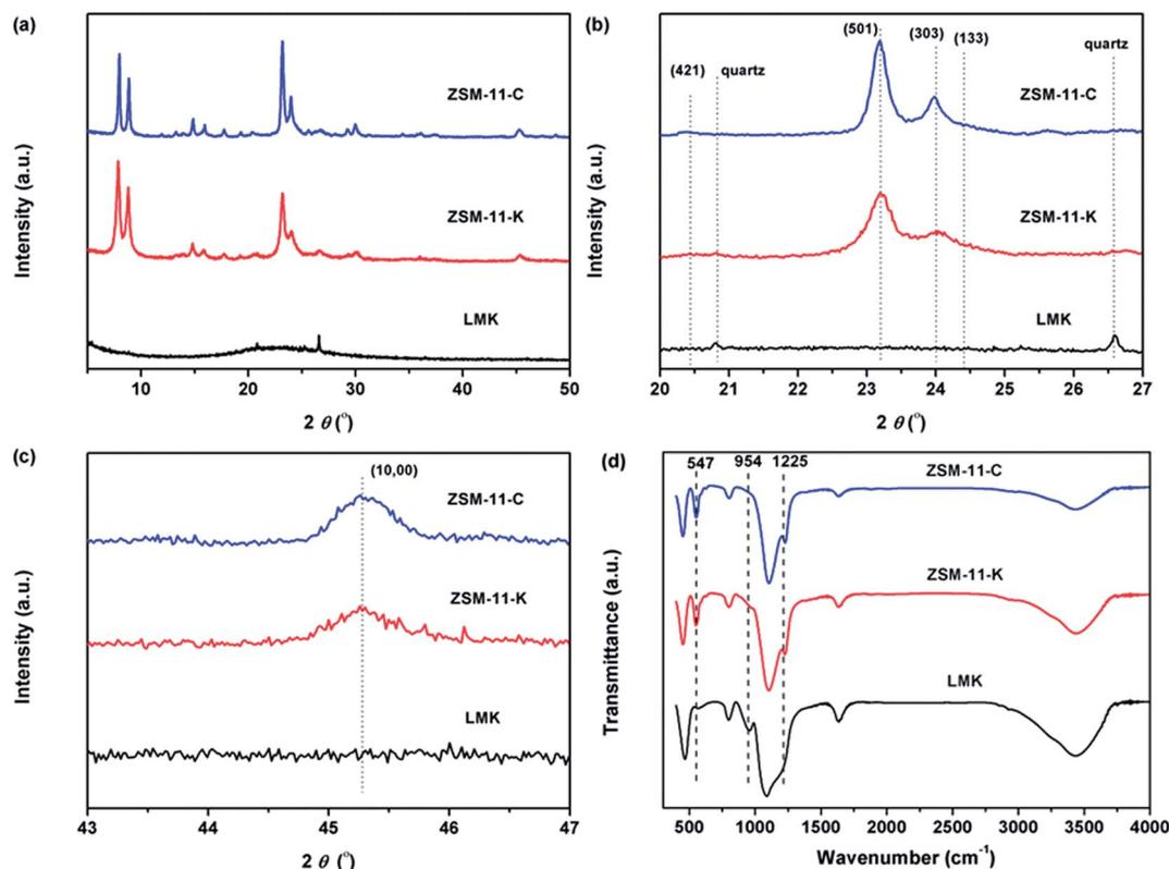
Fig. 2 (a) XRD pattern, (b) enlarged  $2\theta$  region from  $20^\circ$  to  $27^\circ$ , (c) enlarged  $2\theta$  region from  $43^\circ$  to  $47^\circ$ , and (d) FTIR spectra of LMK, ZSM-11-C and ZSM-11-K.
