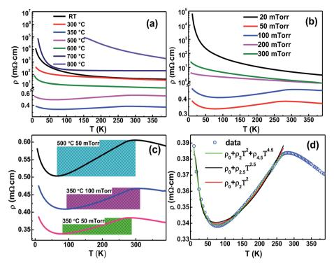
Fig. 5 Resistivity vs. temperature for NCO films grown under (a) different  $T_{\rm G}$  at 50 mTorr  $O_{\rm p}$ , (b) different  $O_{\rm p}$  at 350 °C, (c) temperature window for metallic behavior in the NCO films marked with a rectangle, and (d) simulations on the semiconductor–metal transition of the film fabricated at  $T_{\rm G} = 350$  °C and  $O_{\rm p} = 50$  mTorr.
