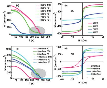
Fig. 9 M-T and FC-ZFC curves of the NCO films grown at different: (a)  $T_{\rm G}$ , and (c)  $O_{\rm p}$ . Hysteresis loops of the NCO films grown at different: (b)  $T_{\rm G}$ , and (d)  $O_{\rm p}$ .
