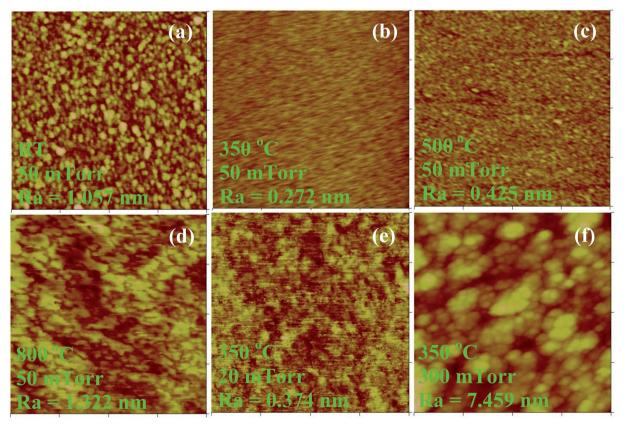
Fig. 4 Surface morphologies of the NCO films grown under different  $T_G$  and  $O_p$  (1  $\times$  1  $\mu$ m<sup>2</sup>).
