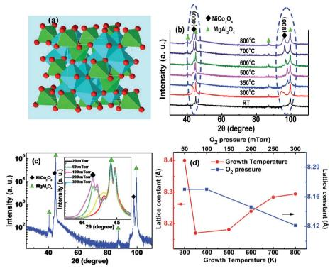
Fig. 1 (a) Schematic of inverse spinel NiCo<sub>2</sub>O<sub>4</sub>, (b) XRD  $\theta$ -2 $\theta$ -scans of the NCO films grown under 50 mTorr  $O_p$  at different  $T_G$ , (c) XRD patterns of the NCO thin films grown under 50 mTorr  $O_p$  at 350 °C, and (d) c-axis lattice parameter dependence on the  $O_p/T_G$ . The inset of (c) is the (400) peaks of the films prepared at different Op at 350 °C.
