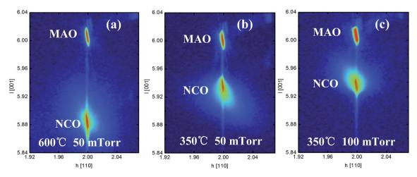
Fig. 2 HR-XRD reciprocal space map around the (226) reflections of the NCO films on MAO substrate grown at (a) 600 °C, 50 mTorr O<sub>D</sub>, (b) 350 °C, 50 mTorr  $O_p$ , and (c) 350 °C, 100 mTorr  $O_p$ .
