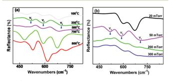
Fig. 7 (a) Infrared spectra of the NCO films grown at different  $T_{\rm G}$  under 50 mTorr  $O_{\rm p}$ , and (b) different  $O_{\rm p}$  at 350 °C.
