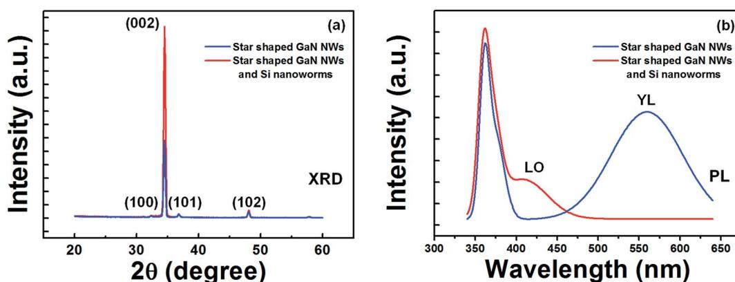
Fig. 3 (a) The XRD patterns for both structures showing the dominant *c*-plane (002) peak position and (b) the PL spectra for both structures showing the dominant band edge emission with YL (for the star-shaped GaN NWs only) and longitudinal phonon recombination (for the hybrid structure).
