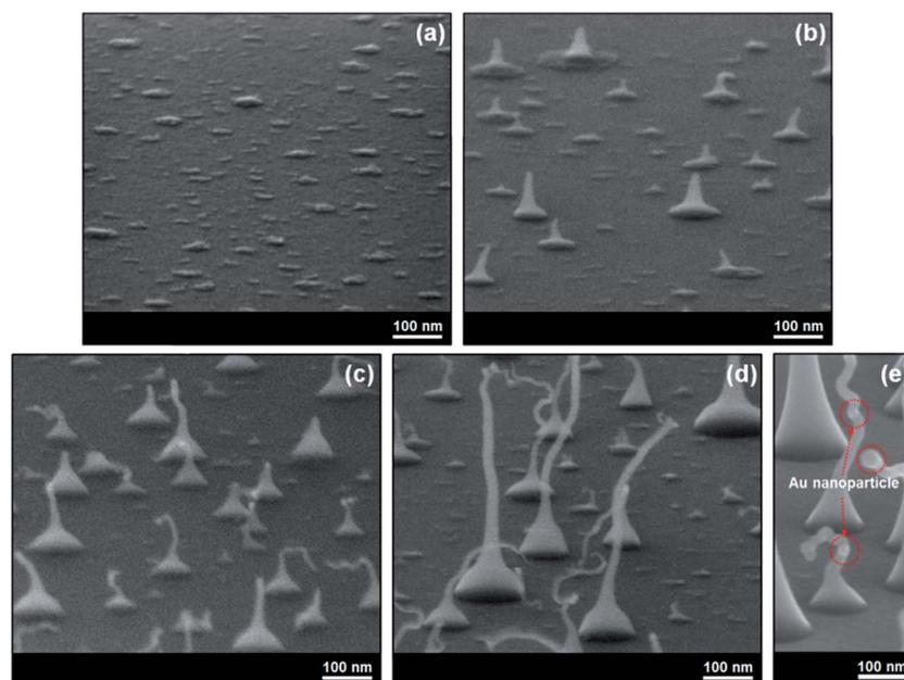
Fig. 6 (a) An FE-SEM image of the island-like seed formation of the Au-Si solid solution. (b) An FE-SEM image at the beginning of the Si nanoworms following the base-growth mechanism. (c) An FE-SEM image of the Si nanoworms showing the drifted Au nanoparticles at the top. (d) An FE-SEM image of the final Si nanoworms structure after 1 h of growth. (e) An FE-SEM image of various Si nanoworms with drifted Au nanoparticles.
