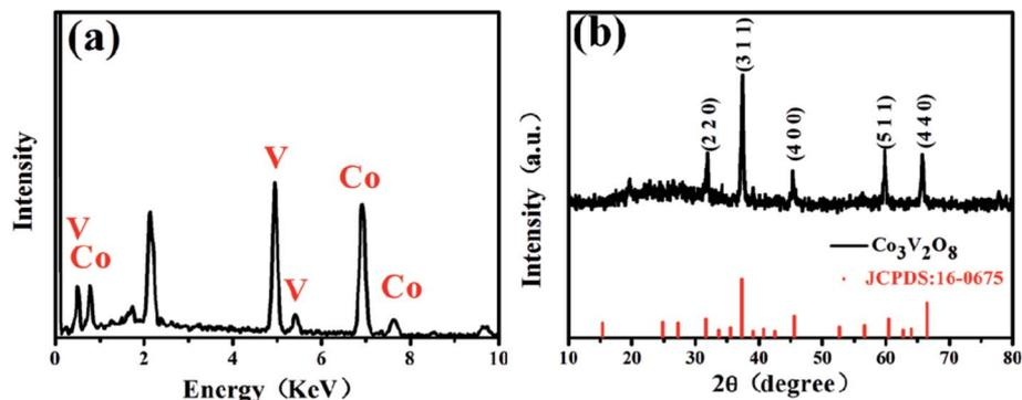
Fig. 1 EDS spectrum (a) and XRD pattern (b) of the obtained  $\text{Co}_3\text{V}_2\text{O}_8$  micro-pencils. EDS spectrum indicates the obtained materials are composed of elements Co, V and O, while the XRD pattern demonstrates the obtained  $\text{Co}_3\text{V}_2\text{O}_8$  micro-pencils have cubic crystal structures (JCPDS no. 16-0675).
