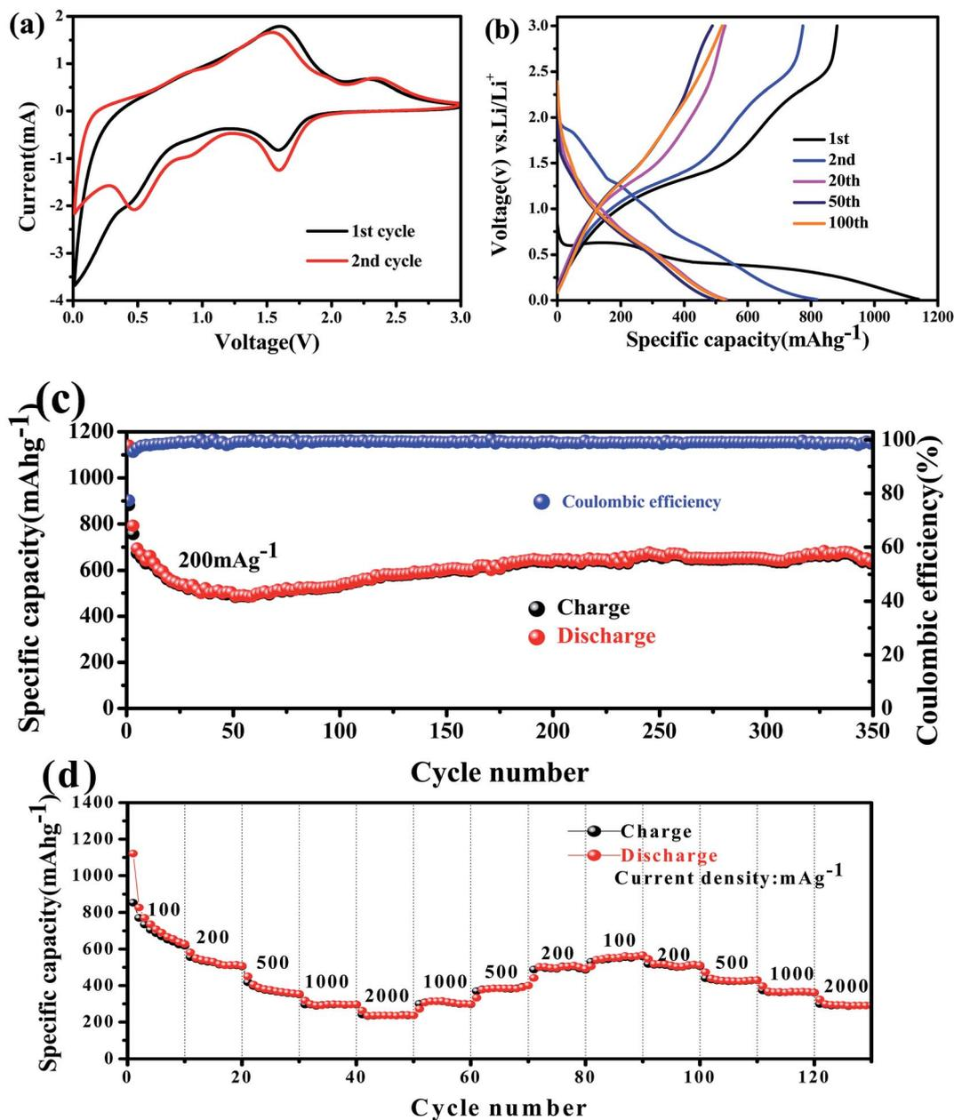
Fig. 5 Electrochemical properties of  $\text{Co}_3\text{V}_2\text{O}_8$  micro-pencils: (a) cyclic voltammogram profiles of the  $\text{Co}_3\text{V}_2\text{O}_8$  micro-pencils; (b) discharge and charge curves at the current density of  $200 \text{ mA g}^{-1}$ ; (c) cycling property at the current density of  $200 \text{ mA g}^{-1}$ , and (d) rate performance at different current densities.
