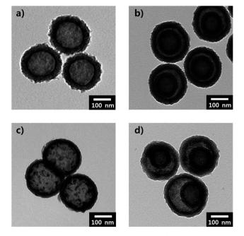
Fig. 2 Transmission electron microscopy (TEM) images of (a) ST SS-HNPs, (b) ST DS-HNPs, (c) NC SS-HNPs, and (d) NC DS-HNPs.
