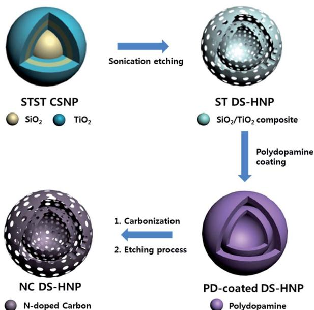
Fig. 1 Schematic illustration of NC DS-HNP synthesis. NC DS-HNPs: nitrogen-doped carbon double-shell hollow nanoparticles; STST CSNPs:  $\text{SiO}_2/\text{TiO}_2/\text{SiO}_2/\text{TiO}_2$  core/shell nanoparticles; ST DS-HNPs:  $\text{SiO}_2/\text{TiO}_2$  double-shell hollow nanoparticles; PD: polydopamine.
