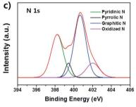
Fig. 5 (a) X-ray photoelectron spectra (XPS) of the NC DS-HNPs and the corresponding high-resolution XPS spectra of (b) C 1s and (c) N 1s features.
