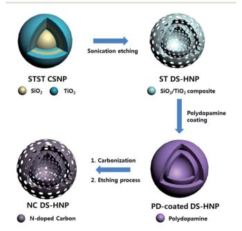
Fig. 1 Schematic illustration of NC DS-HNP synthesis. NC DS-HNPs: nitrogen-doped carbon double-shell hollow nanoparticles; STST CSNPs:  $SiO_2/TiO_2/SiO_2/TiO_2$  core/shell nanoparticles; ST DS-HNPs:  $SiO_2/TiO_2$  double-shell hollow nanoparticles; PD: polydopamine.
