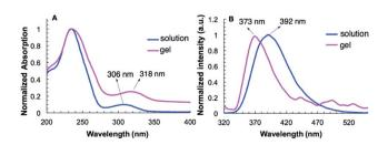
Fig. 2 The (A) absorption (1 mm path length) and, (B) fluorescence emission spectra ( $\lambda_{\text{ex}\_} =$  307 nm) of G2 in water (0.1 mM) and in hydrogel (10 mg mL<sup>-</sup>
