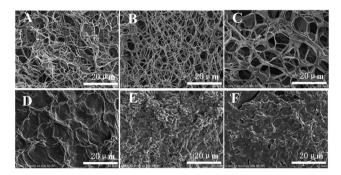
Fig. 1 SEM images of xerogel prepared from the gels of G2 (25 °C) with: (A) water (10 mg mL $^{-1}$ ); (B) water (10 mg mL $^{-1}$ ) with 5  $\mu$ L of added HCl (1 M), followed by regenerating gel after adding 5 μL of Et<sub>3</sub>N; (C) water (10 mg mL<sup>-1</sup>) with 5  $\mu$ L of added CH<sub>3</sub>COOH, followed by regenerating gel after adding 5  $\mu$ L of Et<sub>3</sub>N; (D) benzene (15 mg mL<sup>-1</sup>); (E) toluene (15 mg mL $^{-1}$ ); (F) ethyl acetate (15 mg mL $^{-1}$ ).
