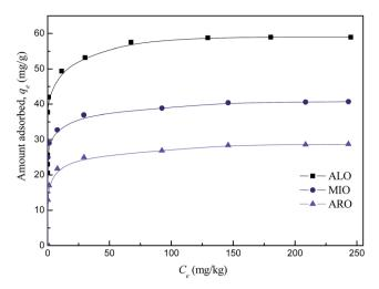
Fig. 5 Equilibrium adsorption isotherms of DBT on the FPC-1 in ALO, ARO and MIO, respectively.
