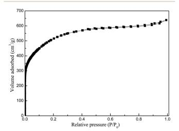
N<sub>2</sub> adsorption isotherms of FPC-1 sample at 77 K.
