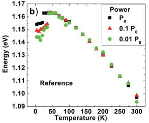
Fig. 2 (a) PL spectra for reference sample from 4–300 K. Inset: Magnification of the PL spectra at low temperatures (T < 100 K) reveals marked diminution in peak at ( $E_{loc}$ ) with increasing T. The small dip at 1075 nm is an artifact due to a grating response. (b) Energy of the highest intensity feature in each PL spectrum as a function of temperature for the different excitation powers.  $P_0$  corresponds to 13 kW cm<sup>-2</sup>.
