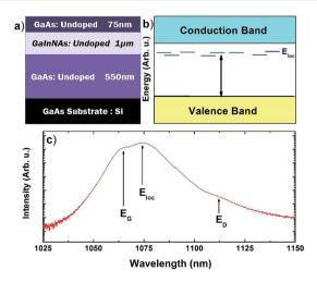
Fig. 1 (a) Schematic of GalnNAs double heterostructure sample (b) qualitative energy location of localized states due to alloy fluctuations ( $E_{\rm loc}$ ) (dashed lines). (c) Example PL spectrum at 4 K of the unhydrogenated reference sample showing two main peaks: at the band gap ( $E_{\rm G}$ ) and the localized states ( $E_{\rm loc}$ ).
