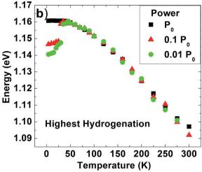
Fig. 3 (a) PL spectra for highest hydrogenated sample as a function of temperature, no attenuation. Inset: Magnification of the PL spectra at low temperatures ( $T < 100\,$  K). (b) Re-emergence of the s-shape temperature dependence with decreasing excitation intensity.  $P_0$  corresponds to 13 kW cm $^{-2}$ .
