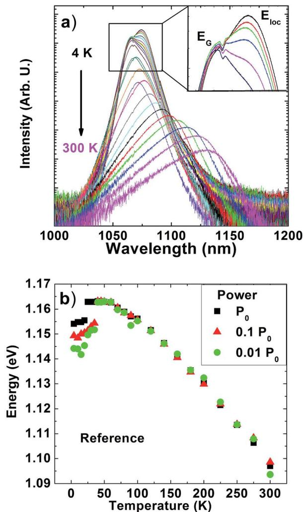
Fig. 2 (a) PL spectra for reference sample from 4–300 K. Inset: Magnification of the PL spectra at low temperatures ( $T < 100$  K) reveals marked diminution in peak at ( $E_{\text{loc}}$ ) with increasing  $T$ . The small dip at 1075 nm is an artifact due to a grating response. (b) Energy of the highest intensity feature in each PL spectrum as a function of temperature for the different excitation powers.  $P_0$  corresponds to 13  $\text{kW cm}^{-2}$ .
