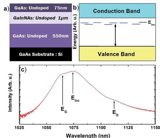
Fig. 1 (a) Schematic of GaInNAs double heterostructure sample (b) qualitative energy location of localized states due to alloy fluctuations ( $E_{loc}$ ) (dashed lines). (c) Example PL spectrum at 4 K of the unhydrogenated reference sample showing two main peaks: at the band gap ( $E_G$ ) and the localized states ( $E_{loc}$ ).
