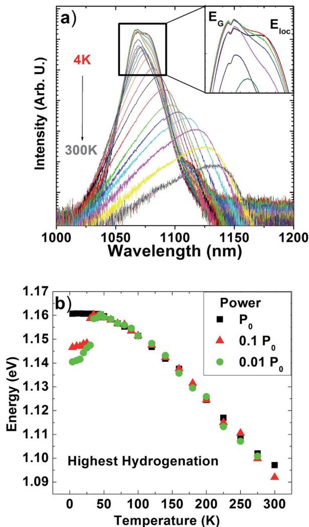
Fig. 3 (a) PL spectra for highest hydrogenated sample as a function of temperature, no attenuation. Inset: Magnification of the PL spectra at low temperatures ( $T < 100$  K). (b) Re-emergence of the s-shape temperature dependence with decreasing excitation intensity.  $P_0$  corresponds to  $13 \text{ kW cm}^{-2}$ .
