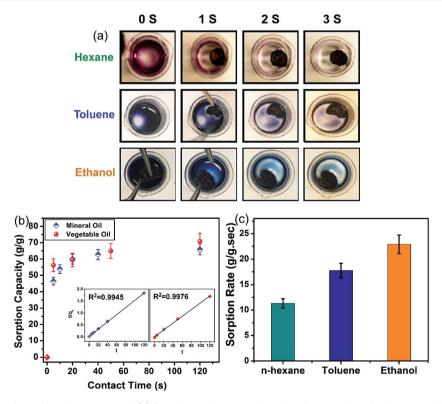
Fig. 4 Kinetics of the sorption of graphene aerogel. (a) Experimental system showing the sorption of n-hexane, toluene and ethanol by the graphene aerogel within 3 seconds, (b) oil uptake experiment using the graphene aerogel shows that the sorption reaches its maximum saturation level within 1 minute for mineral oil and vegetable oil (inset shows the linear fit of the experimental data to the pseudo second order kinetic model for both oils) and (c) average sorption rate of the organic solvents
