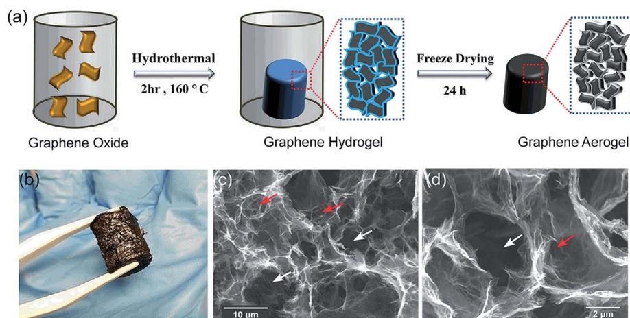
Fig. 1 Graphene aerogel synthesis and its morphology. (a) Schematic showing the experimental steps and synthetic conditions using graphene oxide as the precursor, (b) sample optical image illustrating the foam-type structure of the GA with good mechanical strength and (c and d) SEM images showing that graphene sheets are interconnected in a random fashion to form a three dimensional porous structure with pores of various sizes and shapes.
