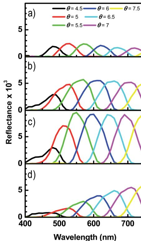
Fig. 6 Spectra of light diffracted by the fringes shown in Fig. 2 of the (a) [Au] = 32, (b) [Au] = 40, (c) [Au] = 52 and (d) [Au] = 60 samples. Incident angle was set to  $30^\circ$  and the diffracted angle ( $\theta$ ) refer to the specular reflection.
