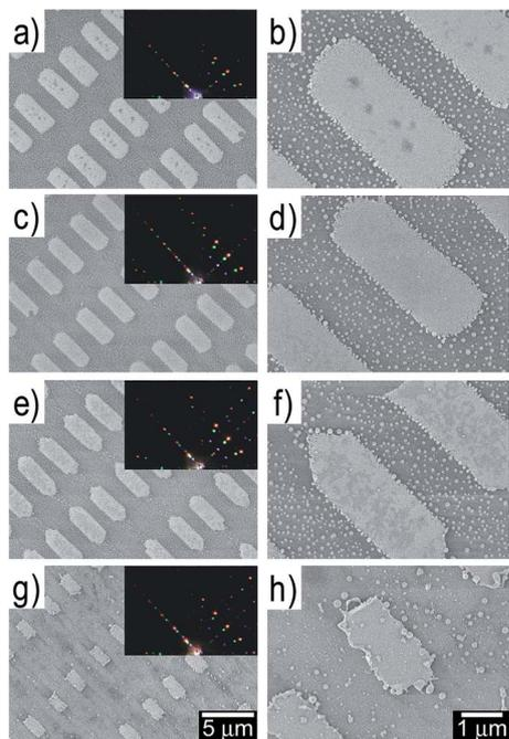
Fig. 5 SEM images of the same 2D pattern of the (a, b) [Au] = 32, (c, d) [Au] = 40, (e, f) [Au] = 52 and (g, h) [Au] = 60 samples. SEM images of the same column have the same magnification and images in the same row refer to the same pattern. Insets in the left column images show the diffraction pattern of the corresponding periodic structure.
