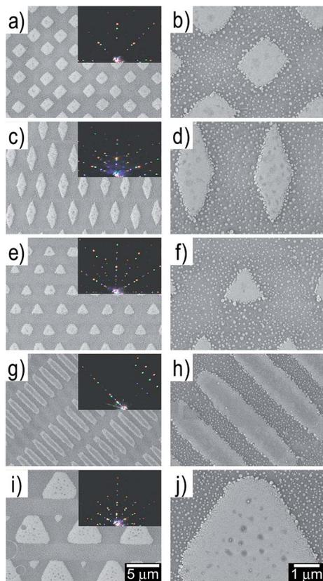
Fig. 4 SEM images of 2D patterns of the  $[Au] = 32$  sample. SEM images of the same column have the same magnification and images in the same row refer to the same pattern. Insets in the left column images show the diffraction pattern of the corresponding periodic structure.
