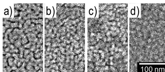
**Fig. 1** SEM images of as grown regions for the samples having (a) [Au] = 32, (b) [Au] = 40, (c) [Au] = 52 and (d) [Au] = 60.
