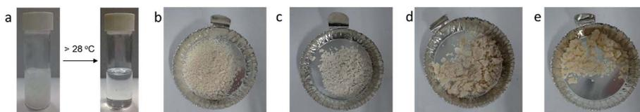
Fig. 3 Appearance of paraffin and ODA/MMT absorbed paraffin with different absorption efficiencies: (a) paraffin, the organoclays absorbed paraffin at (b)  $\eta_{\text{C}_{18}} = 0.26$ , (c)  $\eta_{\text{C}_{18}} = 1.2$ , (d)  $\eta_{\text{C}_{18}} = 2.5$ , and (e)  $\eta_{\text{C}_{18}} = 4.5$ .
