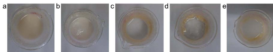
**Fig. 1** Appearance of Na<sup>+</sup>-MMT clay intercalated with different equivalent ratios of ODA-salts at (a) 0 CEC or without ODA, (b) 0.5 CEC, (c) 1.0 CEC, (d) 1.5 CEC, and (e) 2.0 CEC.
