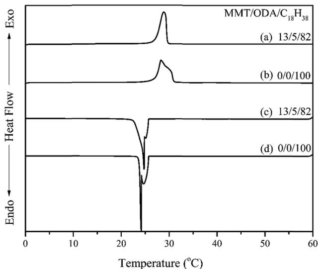
Fig. 4 DSC curves of MMT/ODA/C<sub>18</sub>H<sub>38</sub> at 13/5/82 weight ratio vs. C<sub>18</sub>H<sub>38</sub> under temperature scanning between 0 °C and 60 °C.
