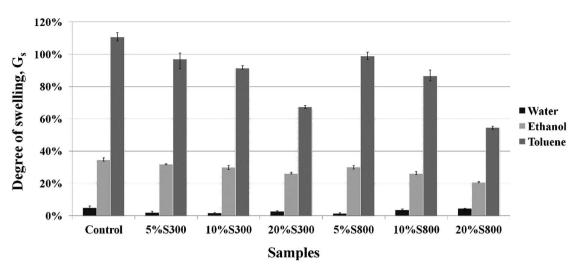
Fig. 9 Degree of swelling of the thermoset composites in water, ethanol and toluene after 24 h.
