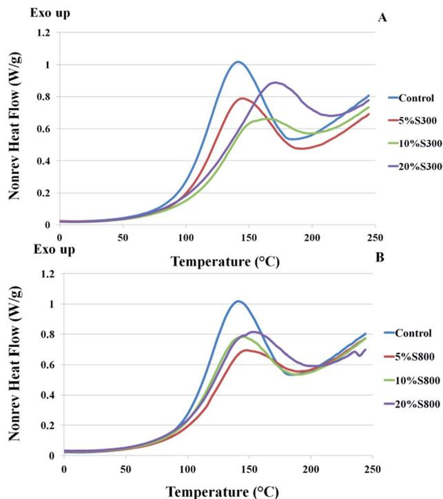
Fig. 4 DSC thermograms of formulations comprised of ELO, Pripol, DMAP and different amounts of S300 (A) and S800 (B) – 5, 10 and 20%wt.
