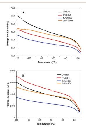
Fig. 7 Storage modulus of the thermoset films with S300 (A) and S800 (B) at different loadings - 5, 10, 20 wt% as a function of temperature.
