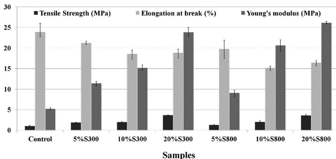
Fig. 8 Mechanical properties of the thermoset composites.
