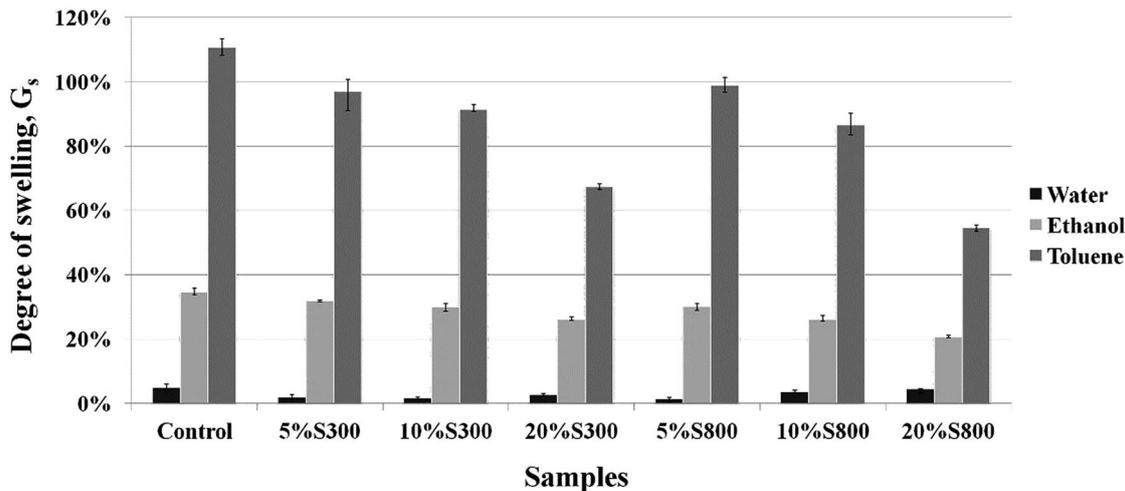
Fig. 9 Degree of swelling of the thermoset composites in water, ethanol and toluene after 24 h.
