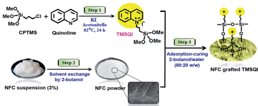
Scheme 1 Schematic of the synthesis of TMSQI and its grafting onto the surface of NFC in 2-butanol/water.
