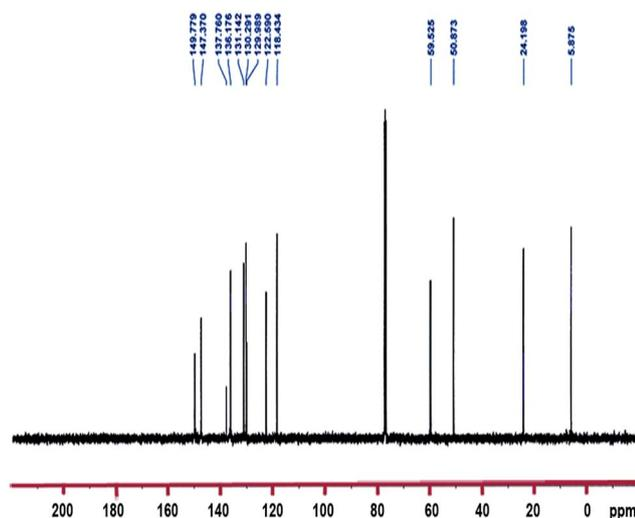
Fig. 2 <sup>13</sup>C NMR spectrum of TMSQI.
