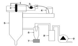
Fig. 1 Experimental apparatus of spray drying: (1) compressed air collection; (2) two-fluid spray nozzle; (3) peristaltic pump; (4) suspension liquid; (5) spray cylinder; (6) cyclone separator; (7) product collecting container; (8) outlet filter; (9) air purge unit.
