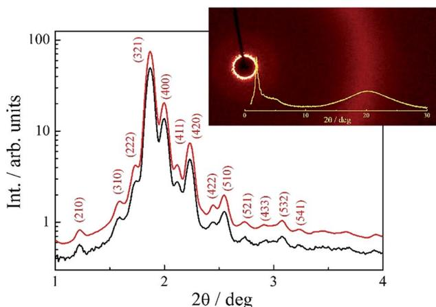
Fig. 5 Low angle X-ray diffractogram (black line) registered for compound **VI.1** at 50 °C. The fitting curve (red line) was obtained assuming crystallographic lattice with  $Im3m$  symmetry and unit cell parameter  $a = 176.8$  Å. In the inset 2D XRD pattern recorded in broad diffraction angle range; diffused high angle signal evidences liquid crystalline character of the phase.
