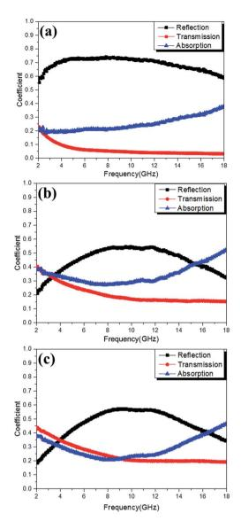
Fig. 12 The reflectance coefficient (R, black curves), transmittance coefficient (T, red curves) and absorption coefficient (A, blue curves) of electromagnetic wave for DSCHP-S14 (a), DSCHP-S23 (b) and DSCHP-S33 (c).
