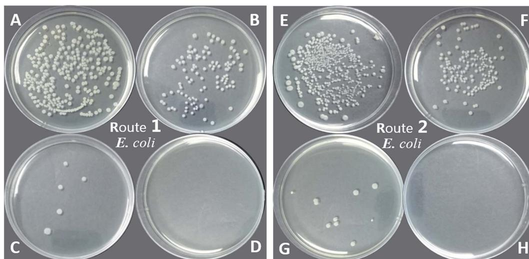
Fig. 10 Anti-microbial activity of PU (blank, A and E), PU-TMG 1 (B), PU-TMG 2 (C), PU-TMG 3 (D) (prepared by route 1), and PU-TMG 1' (F), PU-TMG 2' (G), PU-TMG 3' (H) (prepared by route 2) for *Escherichia coli*.
