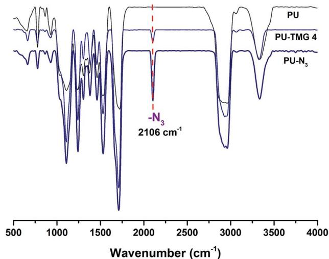
Fig. 4 FT-IR spectra of polyurethane (PU), click-suitable polyurethane (PU-N<sub>3</sub>) and polyurethane with side-chain tetramethylgermanium (PU-TMG 4).
