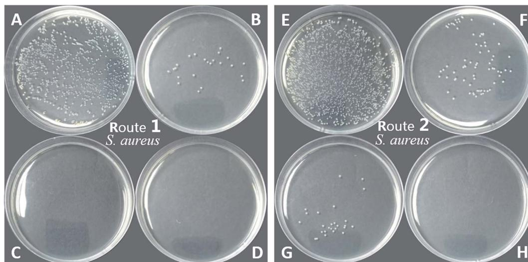
Fig. 9 Anti-microbial activity of PU (blank, A and E), PU-TMG 1 (B), PU-TMG 2 (C), PU-TMG 3 (D) (prepared by route 1), and PU-TMG 1' (F), PU-TMG 2' (G), PU-TMG 3' (H) (prepared by route 2) for *Staphylococcus aureus*.
