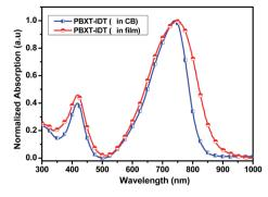
Fig. 1 Absorption spectra of PBXT-IDT in chlorobenzene (CB) and in thin film for comparison.
