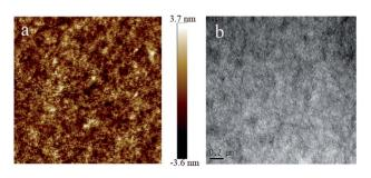
Fig. 6 (a) Tapping mode AFM topography images (2  $\times$  2  $\mu$ m<sup>2</sup>) and (b) TEM image of the P3HT/PBXT-IDT device.
