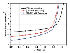
Fig. 4 The  $J\!-\!V$  curves of the all-PSCs based on P3HT/PBXT-IDT mixture.
