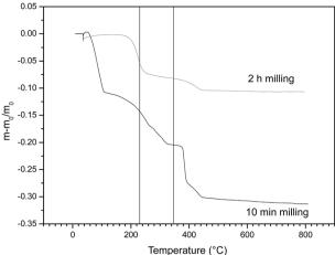
Fig. 6  $\,$  TG patterns of the milled samples (PS 4.29 g, NaOH 1.18 g, HBCD 0.50 q).
