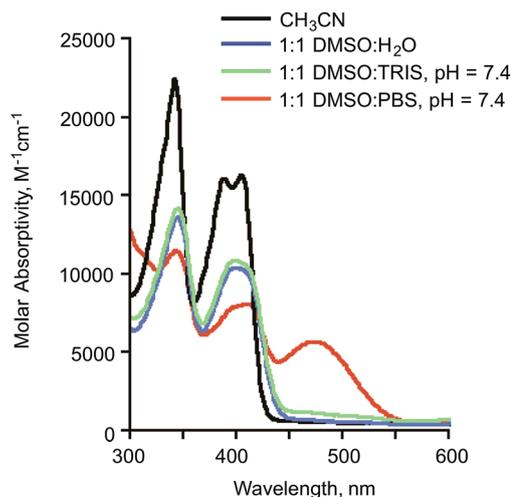
Fig. 3 Absorbance spectra of 2a (0.10 mM) in various solution environments. The ~480 nm absorption feature present in 1 : 1 DMSO : PBS at pH 7.4 is associated with the presence of 2a<sup>-</sup>.
