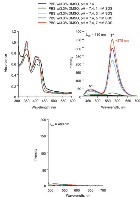
Fig. 8 (a) Absorption spectra of **2a** (0.10 mM) in the presence of various concentrations of SDS. (b) Emission spectra produced with  $\lambda_{\text{ex}} = 410$  nm. (c) Emission spectra produced with  $\lambda_{\text{ex}} = 480$  nm.
