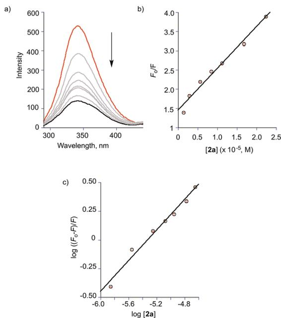
Fig. 10 (a) Fluorescence emission spectra of BSA (1.4  $\mu\text{M}$ ) in the presence of various concentrations of **2a** in TRIS/NaCl : DMSO (96 : 4% v:v, pH = 7.4);  $T = 298\text{ K}$ ,  $\lambda_{\text{ex}} = 282\text{ nm}$ .  $[\mathbf{2a}] = 0, 1.4, 2.8, 5.6, 8.4, 11.2, 16.8, \text{ and } 22.4\ \mu\text{M}$ . (b) Stern–Volmer plot of data for titration of BSA with **2a**. (c) Modified Stern–Volmer plot of data for titration of BSA with **2a**.
