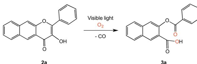
Scheme 1 Visible light-induced CO release reaction of **2a**.
