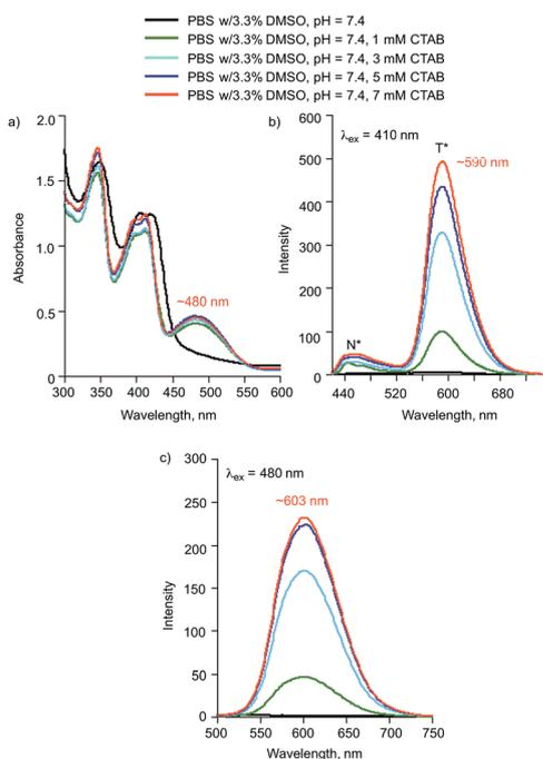
Fig. 7 (a) Absorption spectra of **2a** (0.10 mM) in the presence of various concentrations of CTAB. (b) Emission spectra produced with  $\lambda_{\text{ex}} = 410$  nm. (c) Emission spectra produced with  $\lambda_{\text{ex}} = 480$  nm.
