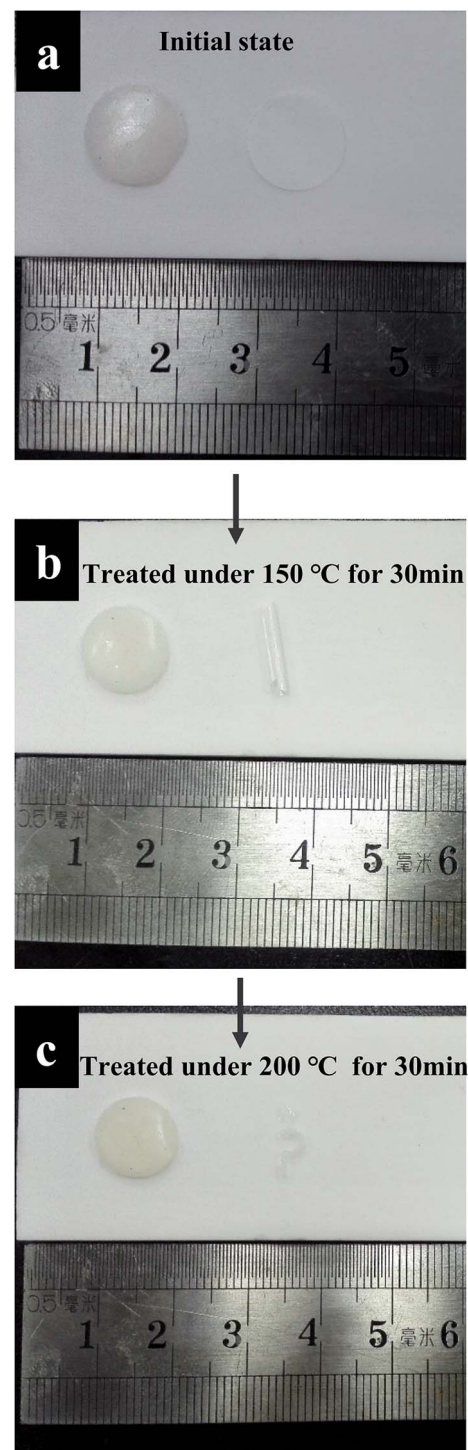
Fig. 2 Photo image of GPE and commercial separator (a) initial state, (b) heat treatment at 150^\circ\text{C} for 30 min and (c) further heat treatment at 200^\circ\text{C} for 30 min.
