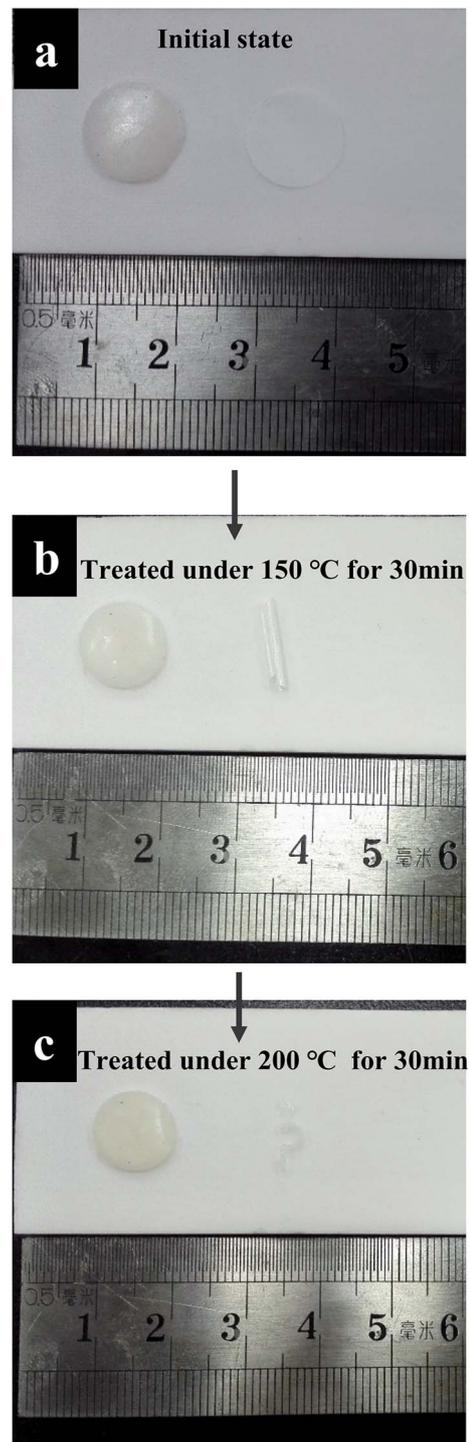
Fig. 2 Photo image of GPE and commercial separator (a) initial state, (b) heat treatment at 150 °C for 30 min and (c) further heat treatment at 200 °C for 30 min.
