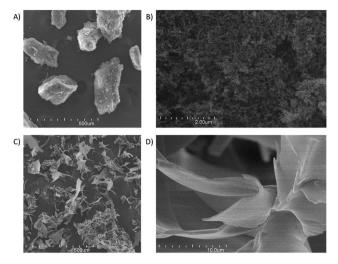
Fig. 8 FE-SEM images of: (A) DCsN at  $100\times$  magnification; (B) DCsN at  $20~000\times$  mag.; (C) LCsN at  $100\times$  mag.; (D) LCsN at  $5~000\times$  mag. All images were acquired with SE detector and 20.0~kV.
