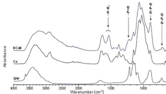
Fig. 4 ATR-FTIR spectra of DCsN, Cs, and TPP.
