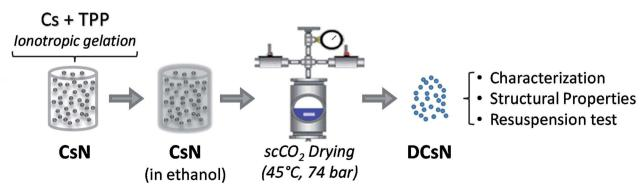
Fig. 1 Experimental scheme for dry Cs nanoparticles production and characterization.
