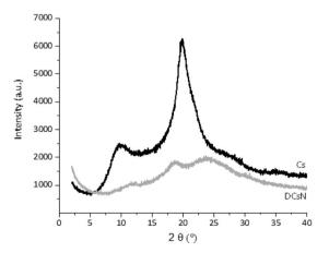
Fig. 6 XRD diffractograms of Cs and DCsN.
