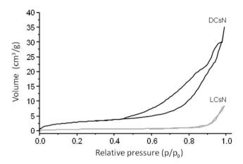
Fig. 7 N<sub>2</sub> adsorption-desorption isotherms of DCsN and LCsN.
