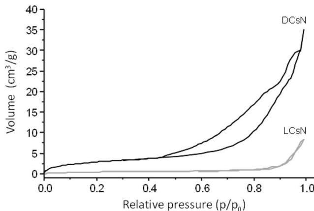
Fig. 7  $\text{N}_2$  adsorption–desorption isotherms of DCsN and LCsN.
