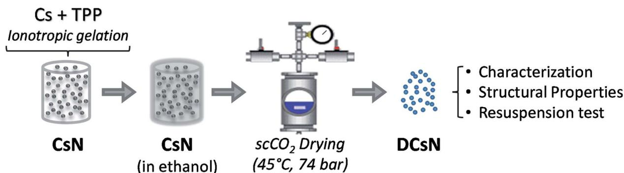
Fig. 1 Experimental scheme for dry Cs nanoparticles production and characterization.
