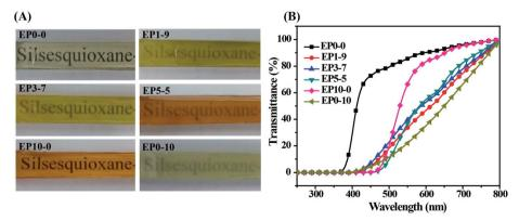
Fig. 1 (A) Photographs and (B) transmittance curves of the cured EP composites.
