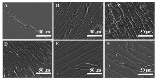
Fig. 2 SEM images of the fracture surfaces of the cured EP composites. (A) EP0-0, (B) EP1-9, (C) EP3-7, (D) EP5-5, (E) EP10-0, (F) EP0-10.
