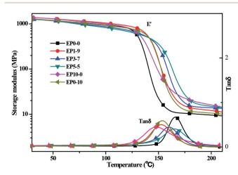
Fig. 3 DMA curves of the cured EP composites.
