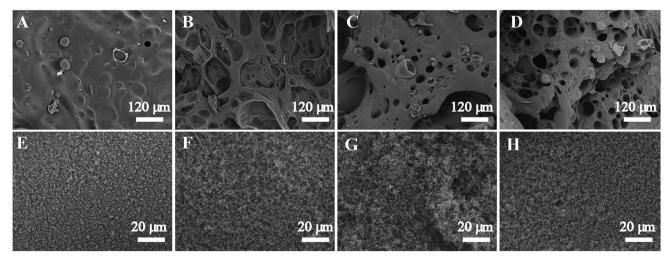
Fig. 6 SEM images of interior char residue of the cured EP composites (top) and SEM images of exterior char residue of the cured EP composites (bottom). (A and E) EPO-0, (B and F) EP5-5, (C and G) EP10-0, (D and H) EPO-10.
