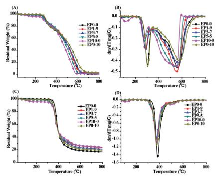
Fig. 4 TGA (left) and DTG (right) curves of the cured EP composites. (A and B) Under air atmosphere, (C and D) under nitrogen atmosphere,  $10 \, ^{\circ}$ C min $^{-1}$ .
